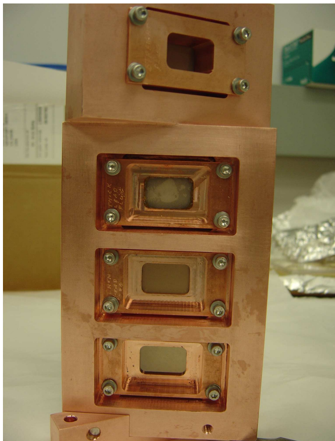
Figure 97: New target design for the 2008 E06-007 run and PREX tests. Beam entrance view with flared windows.
