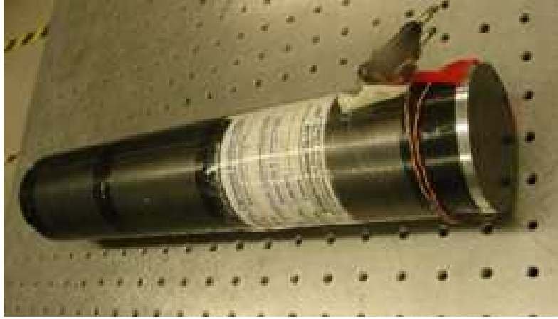
Figure 6: GSO Calorimeter assembled and tested at Carnegie-Mellon University.
