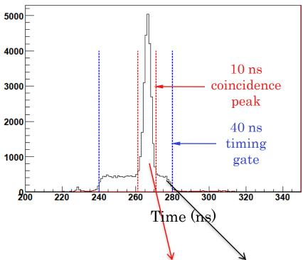
Under test run conditions: signal / background is  $\sim 5/1$ For proposed experiment: signal / background expected to be  $\sim 1/4$ which improves in off-line to  $\sim 12/1$
