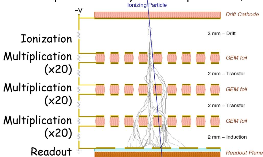
GEM foil: 50  $\mu\text{m}$  Kapton + few  $\mu\text{m}$  copper on both sides with 70  $\mu\text{m}$  holes, 140  $\mu\text{m}$  pitch
