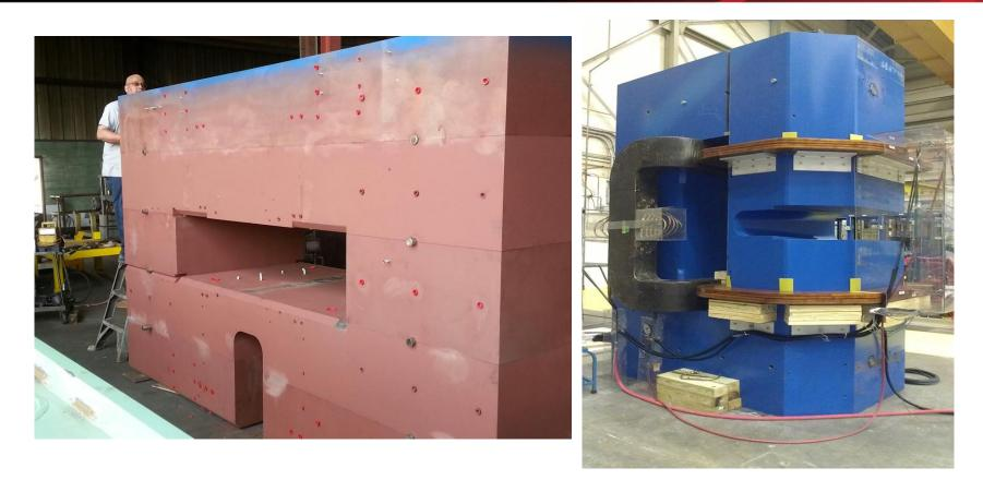
•Magnet Yoke pieces have been machined and delivered.
