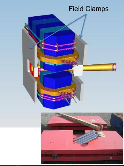
Front field clamps needed to limit target field, less than 40 G.
