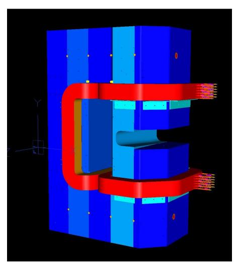
•New racetrack coils allow ease of rotation of magnet and clearance of beam pipe.
