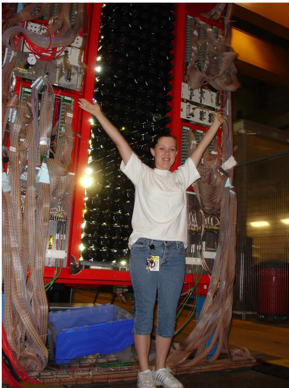
Figure 2: Summer student Emily Sykes (Phebus High School) after she finished re-stacking the refurbished lead-glass shower detectors in the BigBite electron package.
