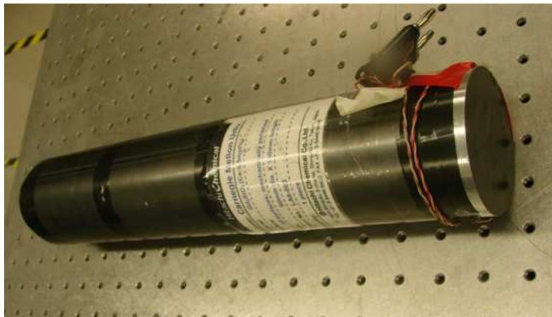
Figure 5: GSO Calorimeter assembled and tested at Carnegie-Mellon University
