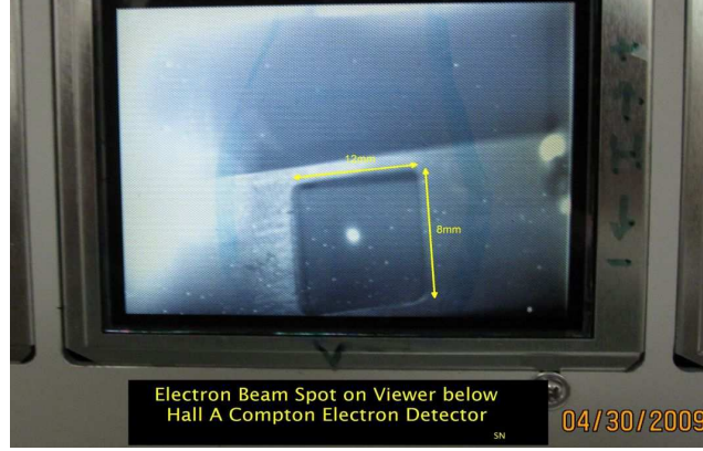
Figure 3: Electron beam spot on the installed Chromax beam viewer confirming the proper installation and alignment of the new electron detector.
