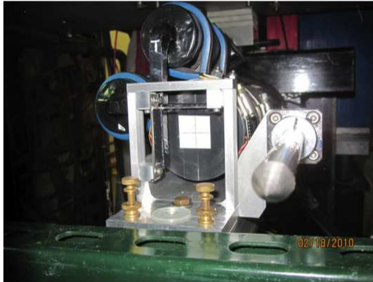
Figure 10: The GSO calorimeter installed in the Hall A Compton Polarimeter
