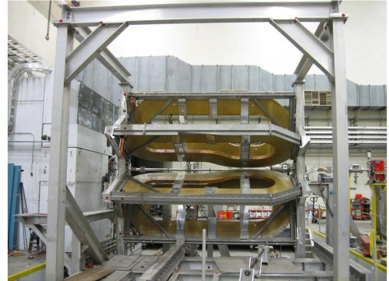
The BLAST spectrometer during disassembly
