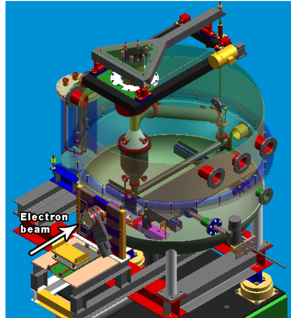
Figure 9: A CAD drawing of the SLAC E158 target chamber. The target loop is remotely movable 6 in in the vertical direction. A table containing optics targets can be moved in and out horizontally.
