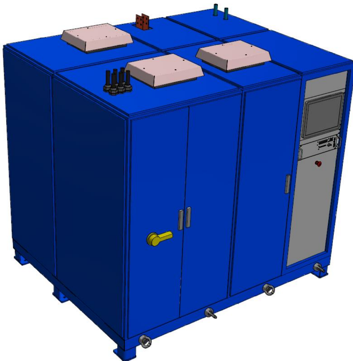
Figure 4 – Preliminary draft of the power converter cabinet
