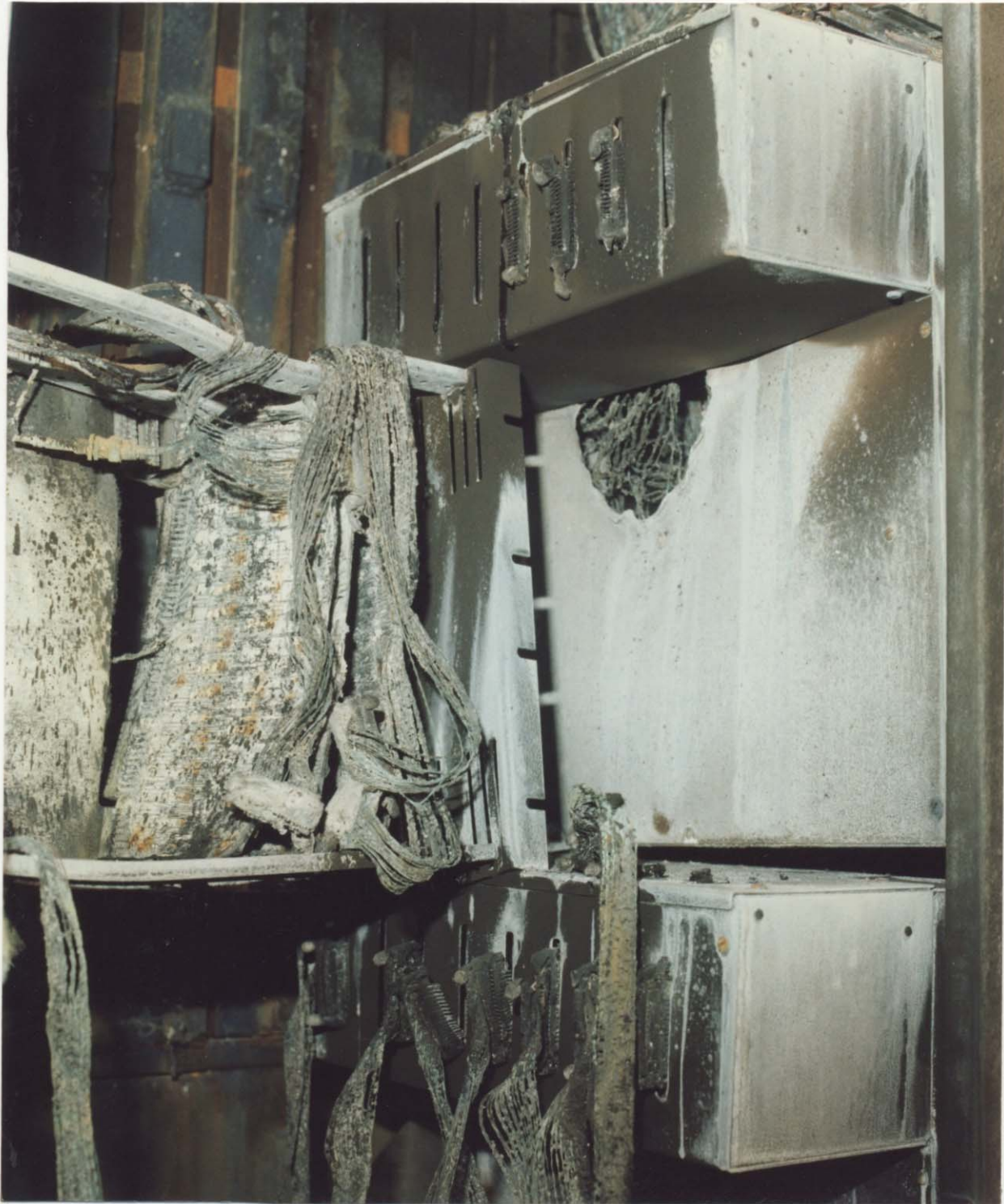
Figure 27. Interior of upstream side of dynode sum box. Connectors handled immediately prior to fire are on lower chassis box. Suspect connector is third from outside.
