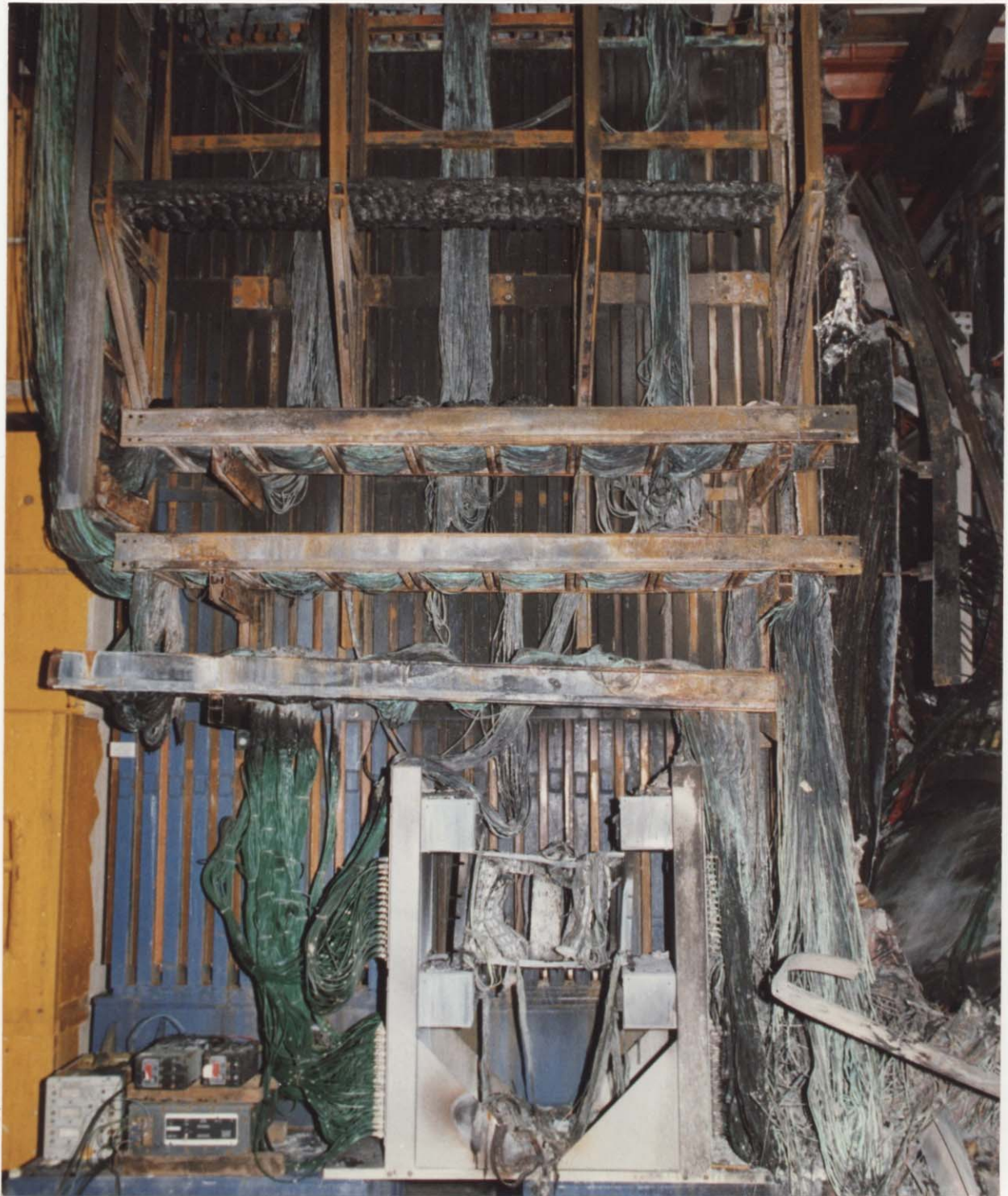
Figure 13. Damage to west side of HC and dynode sum box. Note almost complete destruction of cables on right side of sum box and mostly intact cables on the left.
