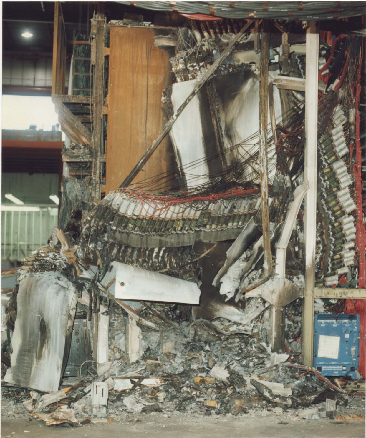
Figure 16. Upstream view of IEC with HxV removed. MF6 is clearly visible on lower right while MF7 is buried under rubble at lower left. Note undamaged cables along east side.
