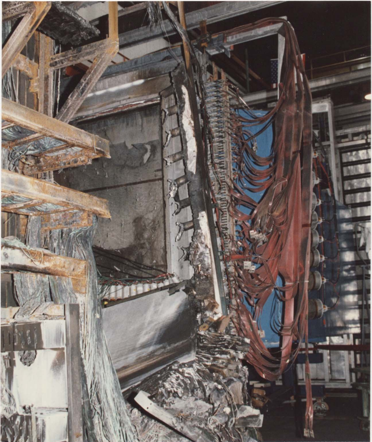
Figure 12. Damage to dynode sum box (with hole burnt through south panel) and IEC second module, remnants of west side of HxV, and damage to P4. Note minor damage to P4 ribbon cables.
