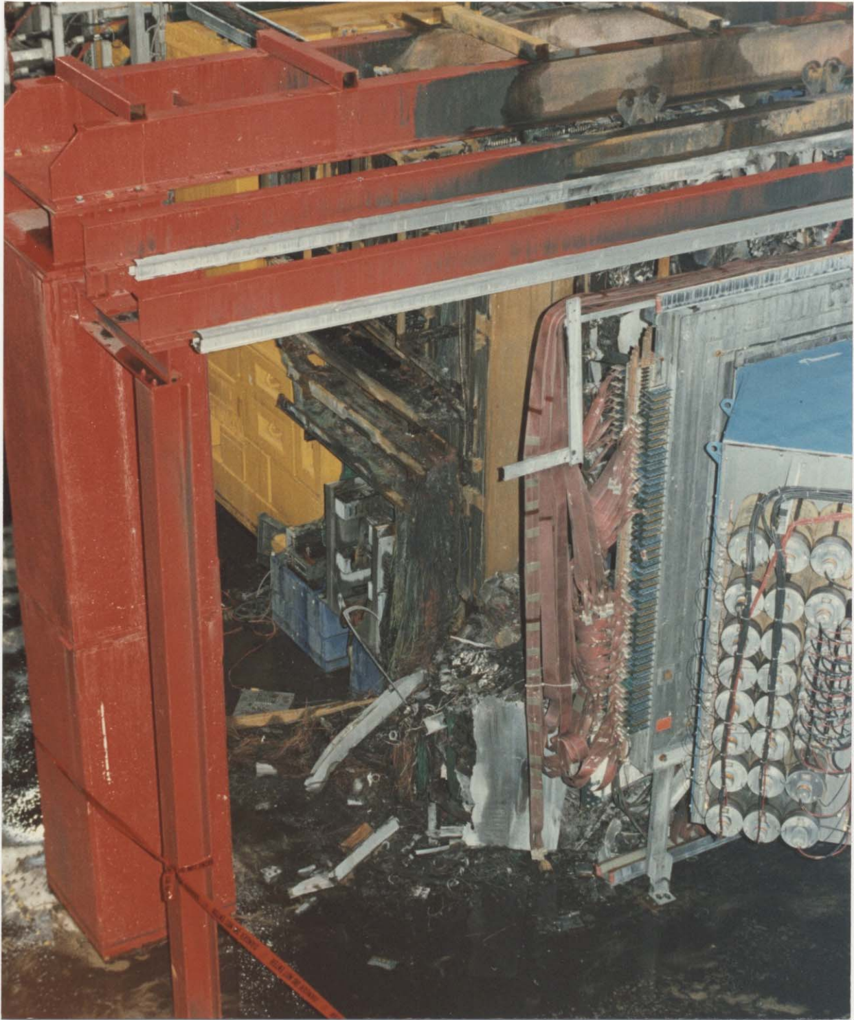
Figure 9. West side of beam line after fire. Note damage to HC, IEC, and support structure, and undamaged ribbon cable on P4.
