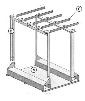
**Step 2: Assemble Beams**
