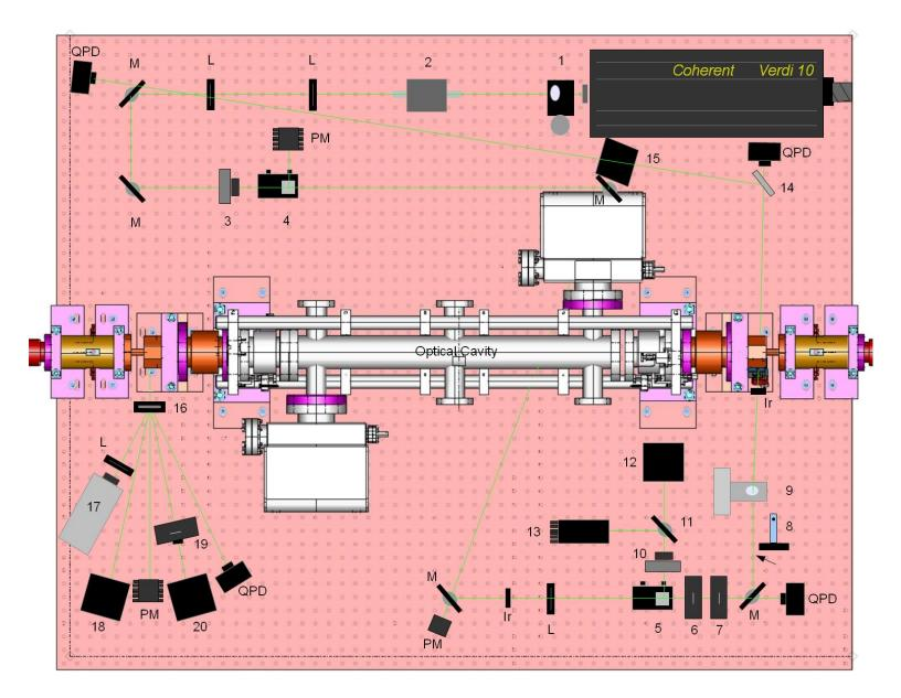
QPD: quadrant photodiode to track laser position
