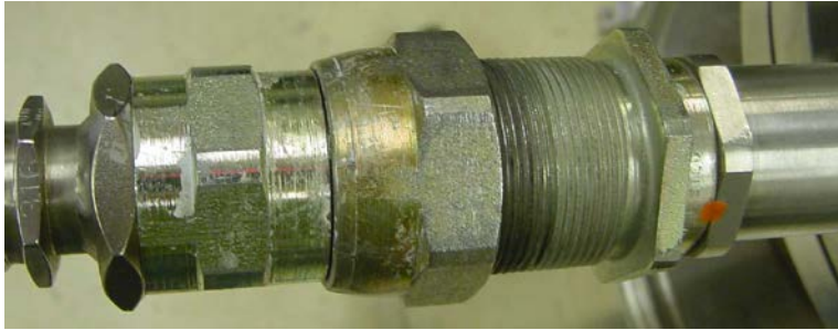
Figure 3 Female to male connection, hand tightened
