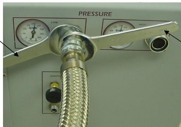
Figure 7-1: Disconnecting flex lines from a compressor package
