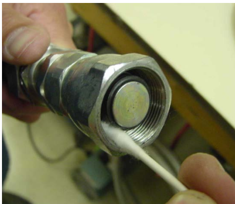
Figure 1 Cleaning the female Aeroquip®
