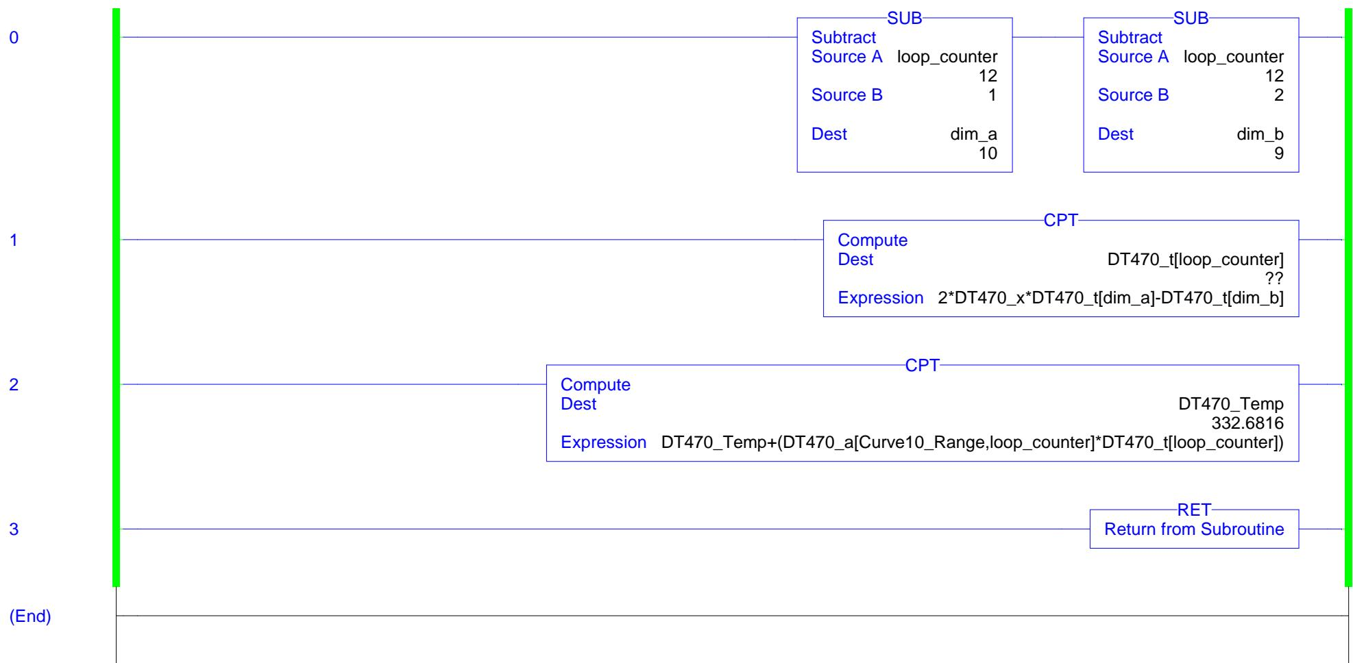
Calculates the temperature of carbon ceramic resistors and temperature diodes.
