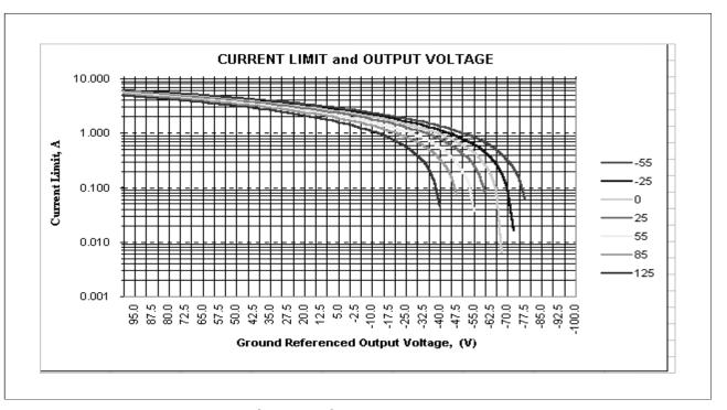
Foldover current limit takes a fraction of the dynamic output voltage (relative to ground where the foldover resistor is connected) and combines it with the static Vbe reference voltage setting current limit. While we often speak of THE current limit, there are actually two, one for the power transistor connected to the positive supply pin and another for the negative side.
