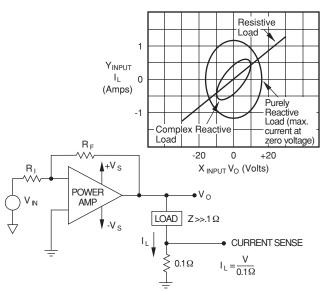
FIGURE 8. AC PDOUT: ELECTRICAL MEASUREMENT
