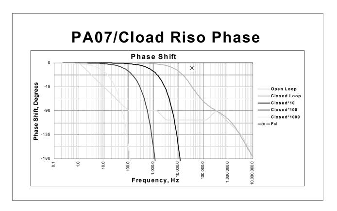
The first thing usually pulled from this graph is phase margin;  $45^{\circ}$  is good,  $30^{\circ}$  is pushing things. Here we see the open loop phase crossing Fcl (closure frequency) at  $107\frac{1}{4}^{\circ}$  (Excel97 gives you the number if you place the cursor on the curve). Phase margin =  $180^{\circ}$  - open loop phase shift, or  $72.75^{\circ}$  in this case.
