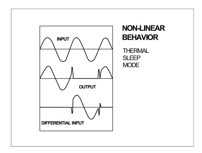
The situation with sleep mode is similar to thermal shutdown. In both cases, the amplifier is disabled by some circuitry which results in the output going into a high impedance state. One additional caution is that when coming out of sleep mode, an amplifier may saturate to one of the rails before recovering.
