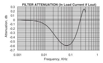
FIGURE 29. DB RESPONSE OF THE MODIFIED MATCHING NETWORK
