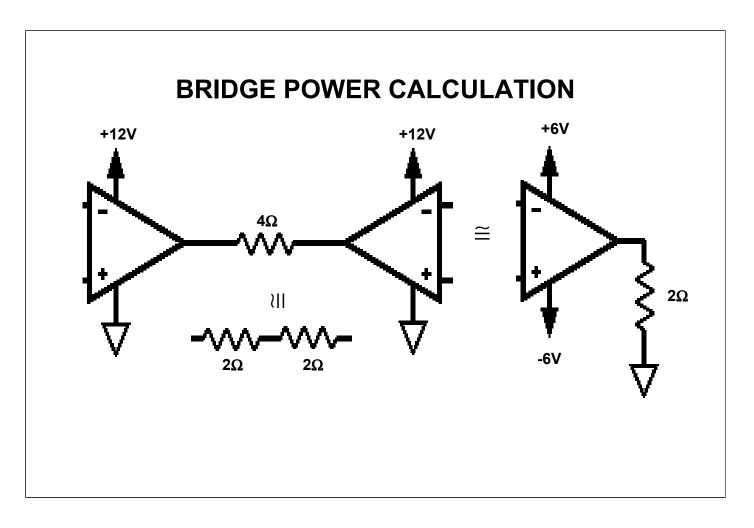
There are several formulae available for calculating worst case power dissipation in a power amplifier (refer to APEX catalog "General Operating Considerations" as well as previous seminar text). These formulae are based on a single power op amp using bipolar, symmetrical supplies. But what about this single supply bridge?
