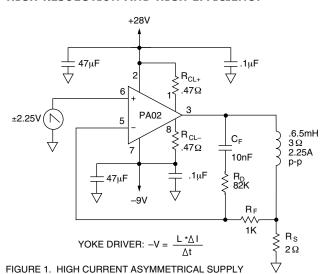
The vertical deflection circuit of Figure 1 was designed to drive a high efficiency RCA CODY II tube. The PA02 was selected for this configuration because of its exceptional linearity and other advantages such as high slew rate, fast settling time, low crossover distortion, and low internal losses. All of these advantages contribute to a
