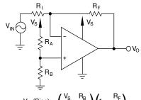
$$\overline{V_{O} \text{ (Bias)}} = \left(\frac{V_{S} - R_{B}}{R_{A} + R_{B}}\right) \left(1 + \frac{R_{F}}{R_{I}}\right)$$
