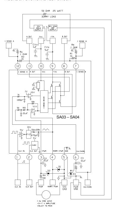
The schematic of Figure 3 can be used to verify the functionality of your amplifier and help you gain a familiarity with proper operation. At either A Out or B Out, with respect to ground, you should observe a square wave approximately 30 V in amplitude with a fixed frequency and duty cycle that varies from approximately 0 to 100% at a rate of 1 Hz. The current limit is set to 2 amps.
