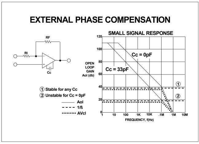
External phase compensation is often available on an op amp as a method of tailoring the op amp's performance for a given application. The lower the value of compensation capacitor used the higher the slew rate of the amplifier. This is due to fixed current sources inside the front end stages of the op amp. Since current is fixed, we see from the relationship of I=CdV/dt that a lower value of capacitance will yield a faster voltage slew rate.
