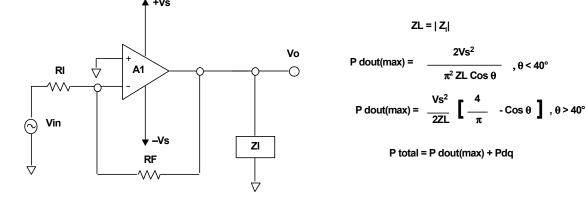
With an AC output and/or reactive loads, output power dissipation calculations can get a bit stickier. Several simplifying assumptions keep the problem reasonable for analysis. The actual internal dissipation can be determined analytically or through thermal or electrical bench measurements. Both Application Note 22 and Application Note 1 General Operating Considerations give details on measuring AC power dissipation.
