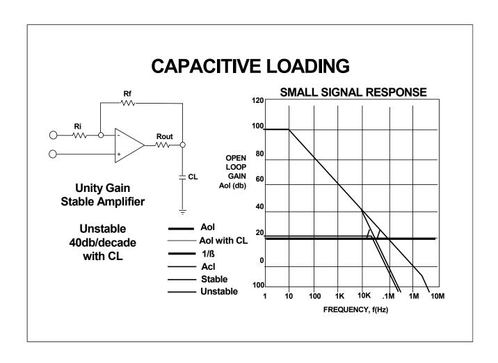
Even when using a unity gain stable amplifier, capacitive loads react with amplifier output impedance, which has the effect of introducing a second pole into the amplifier response which occurs below the unity gain crossover frequency.
