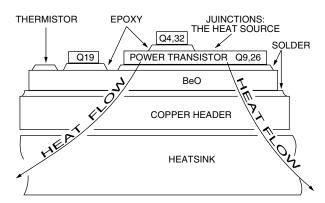
FIGURE 9. THERMO-MECHANICAL DESIGN
