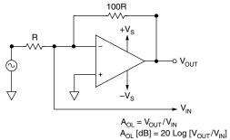
FIGURE 7. OPEN LOOP GAIN
