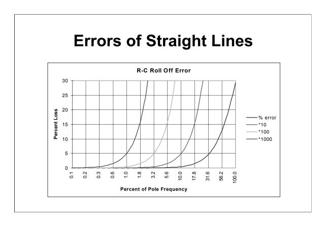
Straight line approximation is a great way to visualize location of corner frequencies but information is lost about attenuation near the corner. In db terms, the errors are small numbers and most circuits have enough frequency margin such that we see no problems.
