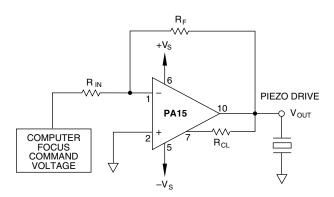
LOW POWER, PIEZOELECTRIC POSITIONING
