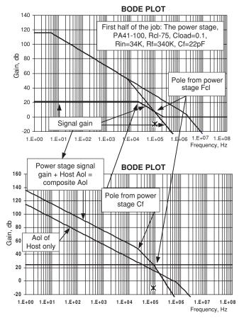
FIGURE 17. A POWER STAGE RESPONSE INCORPORATED INTO A COMPOSITE AMPLIFIER
