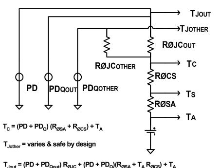
In this model, quiescent power has been split according to the actual transistors generating the heat.  $PD_{Qout}$  is only the quiescent current flowing in the output transistors. When appropriate, this specification will appear in the amplifier data sheet. Multiply this output stage quiescent current times the total supply to find worst case  $PD_{Qout}$
