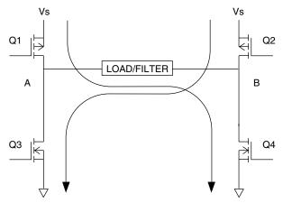
FIGURE 3. BIPOLAR OUTPUT OF THE BRIDGE.
