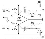
C1 = .1 TO .22  $\mu$ F, CERAMIC DISC C2 = 10  $\mu$ F/AMP OUT (PEAK), ELECTROLYTIC Rs = 3  $-10\Omega$  (PROVISIONAL—HIGHLY INDUCTIVE P.S. LINES)
