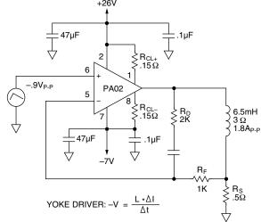
FIGURE 1. HIGH CURRENT ASYMMETRICAL SUPPLY
