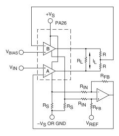
FIGURE 4. ISENSE TRANSCONDUCTANCE BRIDGING AMPLIFIER
