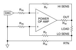
FIGURE 4. REMOTE SENSING PROGRAMMABLE POWER SUPPLY
