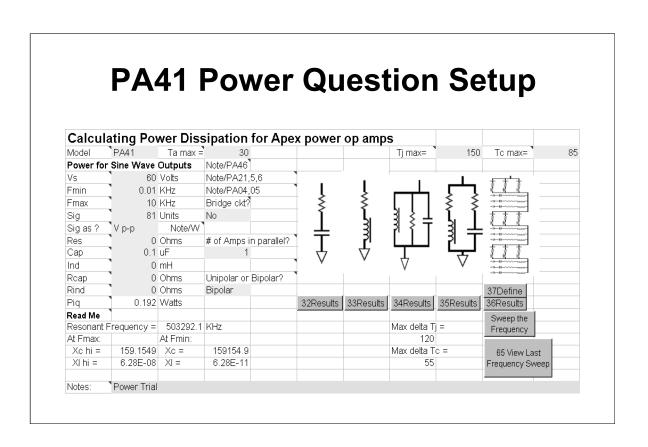
The amplifier selection, load and voltages have all been given. The only frequency that matters is the maximum (no current into a C load at DC). Our stability analysis suggested a maximum of about 10KHz (the Rf-Cf pole frequency).
