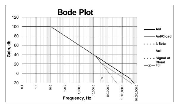
Notice the difference between the curve showing the Signal at Cload and the Acl curve. This is the voltage loss across Riso which is outside the feedback loop and therefore not corrected for amplitude loss. The picture says we really aren't loosing much at usable frequencies. Lets look at another error between 10KHz and closure frequency.
