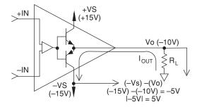
FIGURE 3B. SINKING CURRENT
