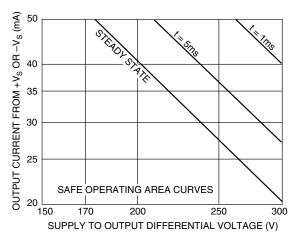
The SOA curves combine the effect of these limits. For a given application, the direction and magnitude of the output current should be calculated or measured and checked against the SOA curves. This is simple for resistive loads but more complex for reactive and EMF generating loads. However, the following guidelines may save extensive analytical efforts:
