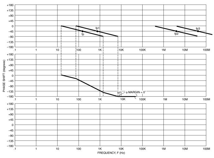
FIGURE 14. OPEN LOOP PHASE PLOT FOR STABILITY CURVE  $\ensuremath{\textcircled{\textcircled{$1$}}}$  (w/o  $\ensuremath{\mbox{R}_{\rm ISO}}$ )
