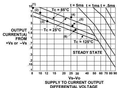
Often the only solution to the conflicting requirement of protection along with reasonable motor acceleration is simply an amplifier with a larger SOA. Not only does the PA61 provide a better SOA fit but the programmable current limit provides additional flexibility in meeting SOA requirements.
