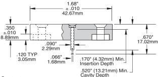
Contacts: Resistance: .020Ω MAX Contact Body: Brass
