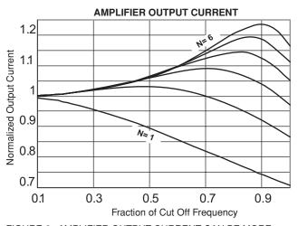
FIGURE 6. AMPLIFIER OUTPUT CURRENT CAN BE MORE THAN EXPECTED
