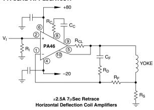
Horizontal deflection amplifiers require both high speed and low distortion. The speed at which current can be changed in a deflection coil is a function of the voltage available from the op amp. In this application an 80 volt power supply is used for the retrace polarity to provide a 7 µSec retrace time, half of which is required for amplifier slewing. This circuit can perform 15.75 KHz deflection in up to 50μH coils at up to 5A p-p.
