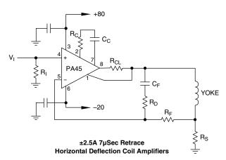
Horizontal deflection amplifiers require both high speed and low distortion. The speed at which current can be changed in a deflection coil is a function of the voltage available from the op amp. In this application an 80 volt power supply is used for the retrace polarity to provide a 7  $\mu$ Sec retrace time, half of which is required for amplifier slewing. This circuit can perform 15.75 KHz deflection in up to  $50\mu$ H coils at up to  $54\mu$ P-p.
