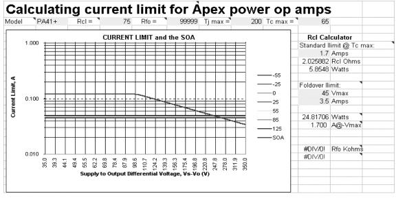
Here we see the difference in limiting on the positive side. While this will not have an effect on driving our normal load because we will calculate this based on the lower negative limit, we will want to know nominal positive limit is about 47mA if any fault conditions must be tolerated.
