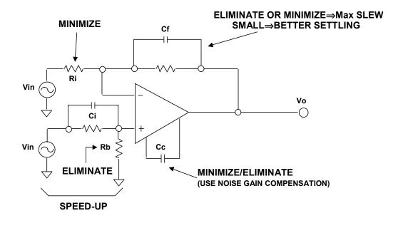
Ever try to buy  $100K\Omega$  coax cable?  $100K\Omega$  could simply not drive the parasitics. So, don't use that impedance trying to deliver input signals to the op amp.
