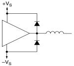
A note of caution about the supply. The energy of the flyback pulse must be absorbed by the power supply. As a result, a transient will be superimposed on the supply voltage, the magnitude of the transient being a function of its transient impedance and current sinking capability. If the supply voltage plus transient exceeds the maximum supply rating or if the AC impedance of the supply is unknown, it is best to clamp the output and the supply with a zener diode to absorb the transient.
