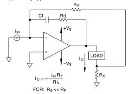
FIGURE 4. CCCS FOR FLOATING LOAD; INVERTING CONFIGURATION
