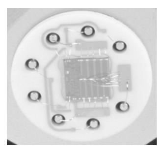
This photo represents the latest technology advance in power op amps. Having only one chip enhances reliability and lowers cost plus enables smaller packages all at the same time. This amplifier is a 150 volt, 5 amp model.
