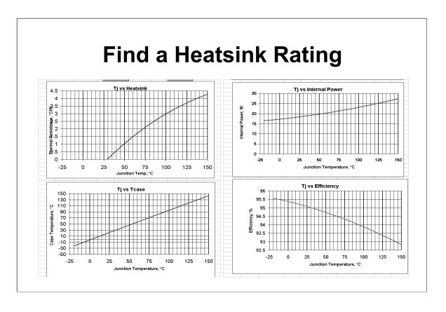
In the upper left graph it looks like a quite small heatsink will keep junction temperatures below maximum. However the graph below says there is little difference between junction and case temperatures and we surely want to keep case temperature a lot lower than 150°C.
