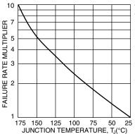
This data was extracted from the base failure rate tables of MIL-HDBK-217C, revision of 1 May 1980.
