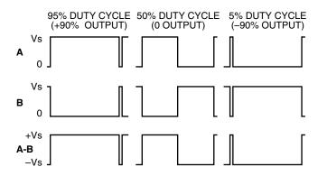
FIGURE 4. H-BRIDGE WAVEFORMS.
