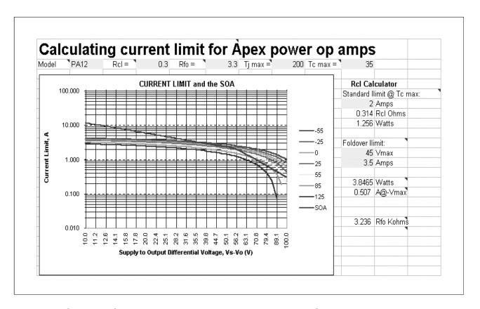
Models featuring foldover current limit may be used in the fixed limit mode by entering ~100Mohms for Rfo. To use foldover enter the desired current limit at 0V output in the RCL calculator and then the desired current limit and voltage when swinging a signal below. If it is possible to meet this slope requirement, a value will be displayed for Rfo. Enter the two resistor values at the top to see the graph. Note that a new Rcl wattage for foldover operation has been calculated.
