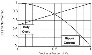
FIGURE 4. DUTY CYCLE AND RIPPLE CURRENT VARIATIONS WITHOUT OUTPUT VOLTAGE
