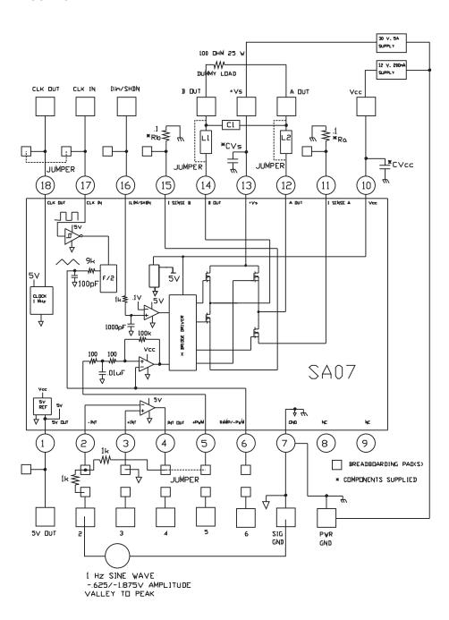
Figure 3 shows a suggested simple test circuit that you can build to gain a familiarity with the evaluation kit as well as the amplifier. At the A OUT or B OUT pads relative to power ground you should observe a square wave with a frequency of approximately 500kHz, 30V p-p which is being modulated from approximately 0 to 100 % duty cycle at a rate of 1 Hz.
