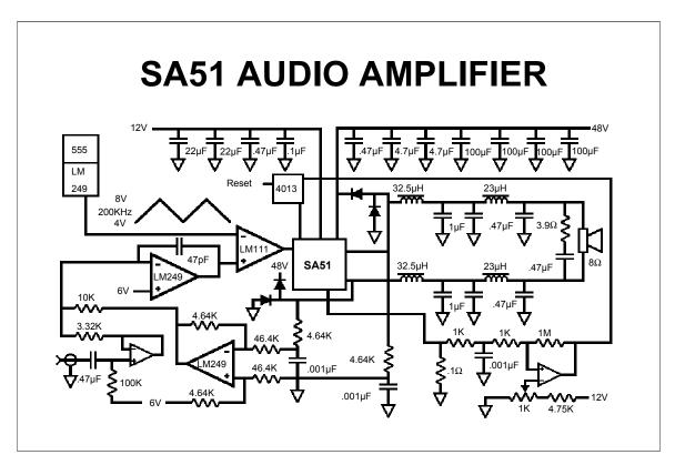
This class "D" audio amplifier is cost effective, cool running, good sounding and delivers up to 100W. Does any one know what this number would be if you bought the equipment as consumer audio gear?
