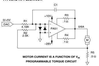
The linear relationship of torque output to current input of the modern torque motor makes this simple control circuit ideal for many material processing and testing applications. The sense resistor develops a feedback voltage proportional to motor current and the small signal properties of the Power Op Amp insure accuracy. With this closed loop operation, temperature induced impedance variations of the motor winding are automatically compensated.
