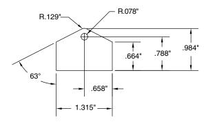
Material: Kapton-MT .002" Thick W/ .0005" thermal compound on each side
