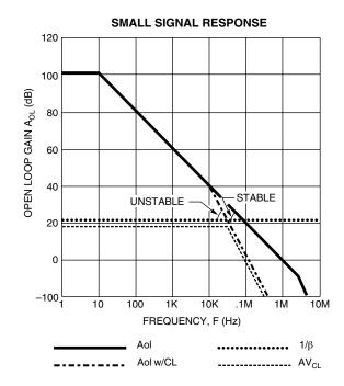
FIGURE 3. CAPACITIVE LOADING
