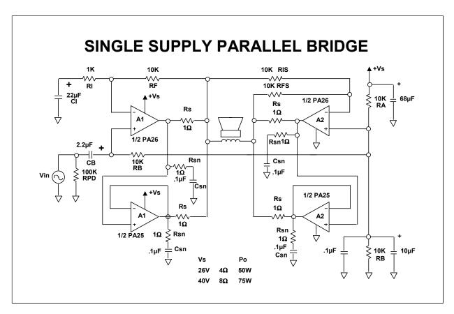
This application utilizes two power op amp circuit tricks—single supply bridge mode to increase output peak-to-peak voltage and parallel power op amps to increase output current.
