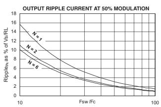
FIGURE 2. OUTPUT RIPPLE CURRENT VARIES WITH ORDER
