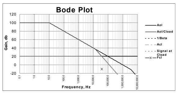
This picture is the first part of the problem. The output impedance of the PA07, plus the current limit resistor along with the big capacitive load, have added an additional pole to the open loop response of the amplifier. This degrades closure rate to 40db per decade--a warning flag. Its too bad we can't use a gain of 100 (40db) where closure rate would have been OK.
