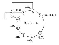
NOTE: Input offset trimpot optional. Recommended value of 100K  $\Omega$ .
