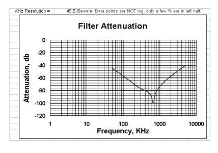
Attenuation is about as expected up to 200KHz, but then the parasitics come into play. We learned earlier that the extremely fast transition times of the PWM amplifiers means high frequency content is powerful well into the megahertz range. This graph is telling us spike content at the filter output is far from ideal. Is this OK? Or should we spend more on better filter components?
