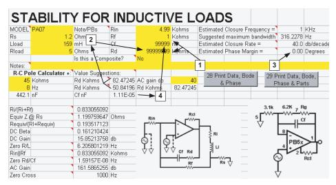
FIGURE 19. STEPS TO STABILITY FOR CURRENT CONTROL WITH INDUCTIVE LOADS
