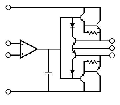
Class "C" output stages tie the bases or gates of the power devices together.
