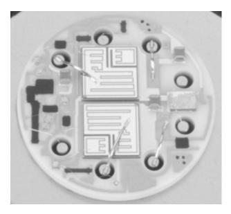
The black areas are thick film resistors which are very cost effective because many resistors can be screened on a single pass and they require no wire bonding. Their intimate contact with the substrate makes them run cool. Wire size here jumps to 10 mils. On higher current products we also use 15 and 20 mil wire.
