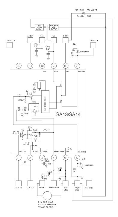
The schematic of Figure 3 can be used to verify the functionality of your amplifier and help you gain a familiarity with proper operation. At Out, with respect to ground, you should observe a square wave approximately 30 V in amplitude with a fixed frequency and duty cycle that varies from approximately 0 to 100% at a rate of 1 Hz.
