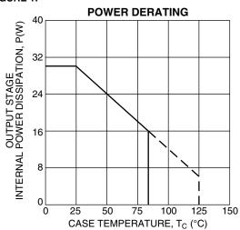
FIGURE 1. PA85 DATA SHEET EXCERPTS
