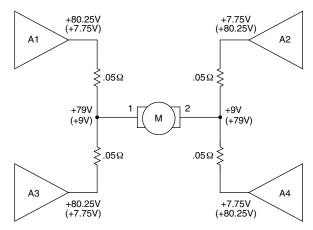
FIGURE 2. FULL SCALE DRIVE VOLTAGES
