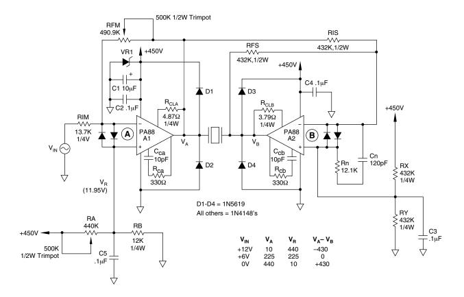
FIGURE 33. 860Vpp PIEZO DRIVE (SINGLE SUPPLY BRIDGE)
