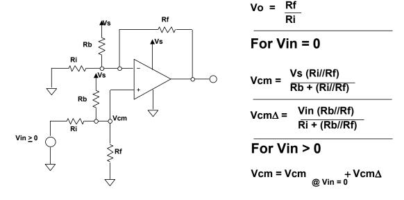
This configuration can easiest be viewed as a differential amplifier with an offset voltage summed in on both + and - input nodes. With this arrangement of resistors the transfer function is: Vout = Rf/Ri Vin.
