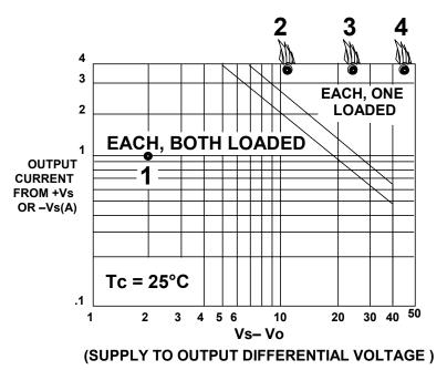
Plotted on the PA21 SOA graph are the four possible operating conditions for the PA21 when used with the Electro-Craft E540.
