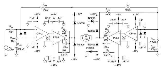
FIGURE 8. PB58A MOTOR DRIVE BRIDGE
