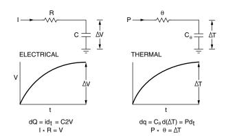
FIGURE 3. ELECTRICAL AND THERMAL MODELS
