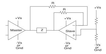
FIGURE 11. THE CLASSIC NON-SYMMETRIC BRIDGE CIRCUIT
