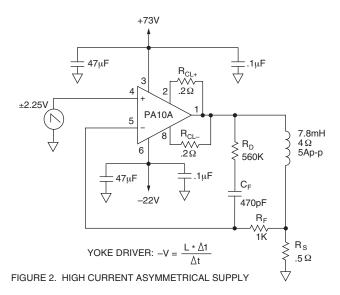
For an even more powerful version of this circuit, the PA10 power op amp can be used, as shown in Figure 2. With this device, a 7.8mH  $4\Omega$  coil can be driven at  $5A_{\text{P-P}}$  with the same timing requirements. Calculations for this design are:
