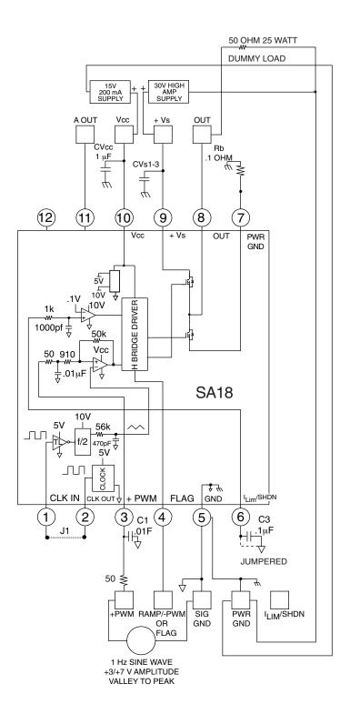
The schematic of Figure 3 can be used to verify the functionality of your amplifier and help you gain a familiarity with proper operation. At Out with respect to ground, you should observe a square wave approximately 30 V in amplitude with a fixed frequency and duty cycle that varies from approximately 0 to 100% at a rate of 1 Hz. The current limit is set to 2 amps.
