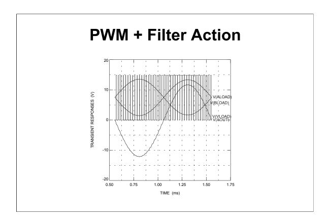
This picture shows the B output, switching at 42KHz, modulated at a 1KHz rate, along with the two filtered outputs and voltage as seen by the load.
