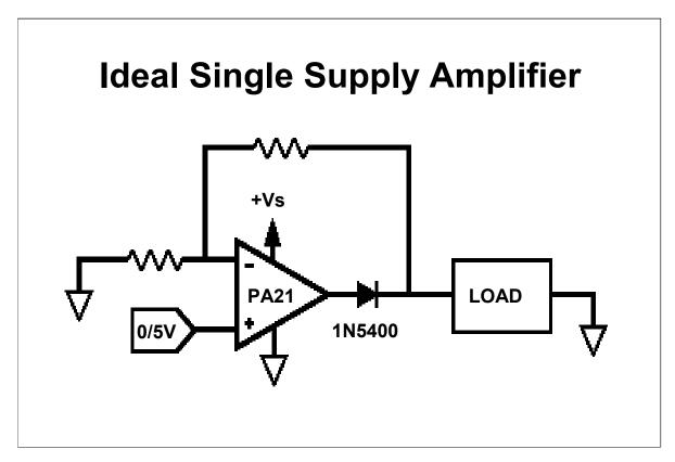
The PA21 series amplifiers feature a common mode voltage range from 0.3V below the negative supply rail (ground in this case) to with in 2V of the positive rail. These amplifiers also swing to about 0.5V of the rail with very light loads making the diode level shifter above quite practical as long as the load is resistive. With the diode inside the feedback loop it contributes essentially no errors at the load.
