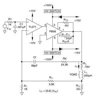
FIGURE 4. ELECTROMAGNETIC DEFLECTION AMPLIFIER
