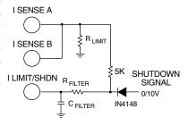
could trip the current FIGURE A. CURRENT LIMIT WITH SHUTDOWN VOLTAGE MODE.
