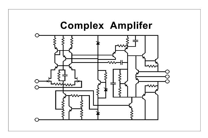
Here is the most difficult and costly way to build a power op amp. Monolithic driver candidates are often lacking in performance above ±15V and above ±40V the picture is down right discouraging.
