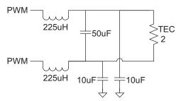
FIGURE 25. A CROSS BETWEEN SPLIT INDUCTOR
