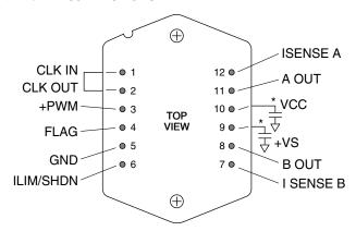
Case tied to pin 5. Allow no current in case. Bypassing of supplies is required. Package is Apex MO-127 (STD). See Outline Dimensions/Packages in Apex data book.
