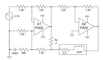
FIGURE 4. ELECTRO-MAGNETIC DEFLECTION (BRIDGE AMPLIFIER)
