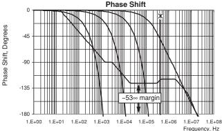
FIGURE 7. AN ISOLATION RESISTOR IS OFTEN THE BEST STABILIZATION METHOD
