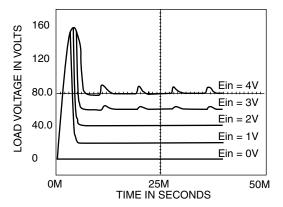
FIGURE 8. TRANSIENT RESPONSE OF LOAD CURRENT WITH FULL WAVE RECTIFIER, C1=1000 μF.
