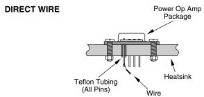
FIGURE 2. MOUNTING TECHNIQUES (CROSS SECTION VIEWS)
