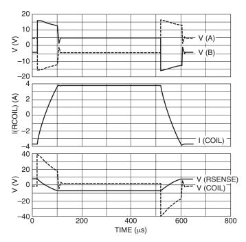
FIGURE 7. BRIDGE DRIVE CURRENTS AND VOLTAGES
