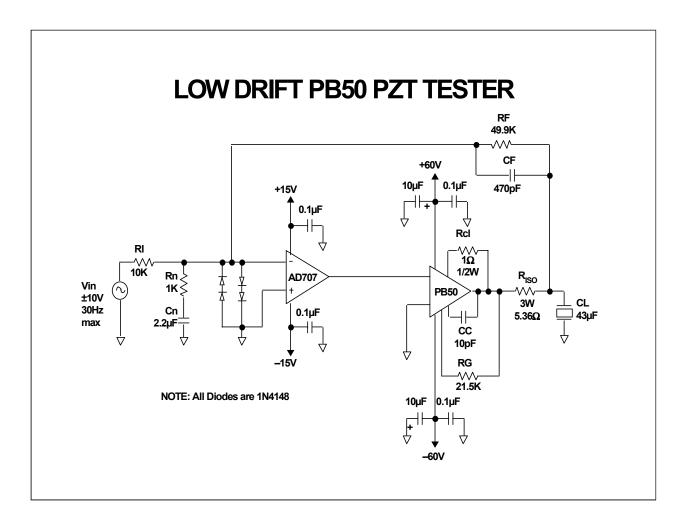
This Low Drift PB50 PZT Tester utilizes the flexibility of the PB58 power booster to provide low drift, high accuracy voltages to the PZT (Piezo Transducer) under test. The AD707 provides a composite amplifier input offset voltage of  $90\mu V$ , and a drift of  $1\mu V/^{\circ}C$ . Higher accuracy can be obtained with a different host amplifier or a better grade of AD707.
