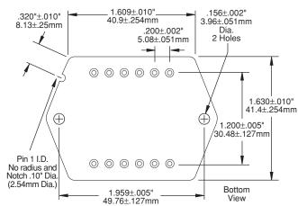
PIN DIAMETER: 1.47/1.57mm or .058/.062" PIN LENGTH: 11.43/12.7mm or .450/.500"
