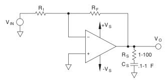
FIGURE 22. OUTPUT R-C-NETWORK ("SNUBBER")
