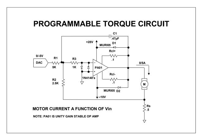
This schematic uses several tricks that we've learned. First of all, notice that the PA01 is operating from non-symmetrical supplies. The –10 volt supply is merely to provide input common mode bias. The 28 volt supply is used to supply the load current.
