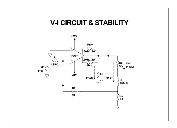
This V-I (Voltage to Current) topology is a floating load drive. Neither end of the load, series RL and LL, is connected to ground.
