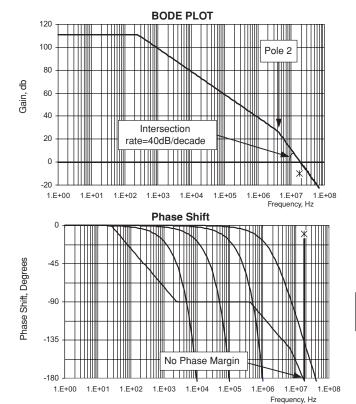
FIGURE 4. ATTEMPTING TO USE AN AMPLIFIER BELOW SPECIFIED MINIMUM GAIN
