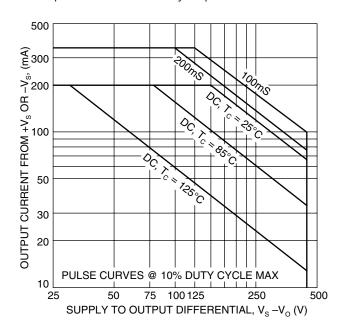
load. This is not the same as the absolute maximum internal power dissipation listed elsewhere in the specification since the quiescent power dissipation is significant compared to the total.
