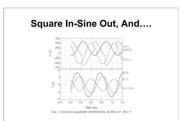
This is a Spice simulation of the previous example showing L1 and C1 stresses when the input signal is a 900Hz, 470V square wave instead of a sine. The modeled filter topology was a dual capacitor design.
