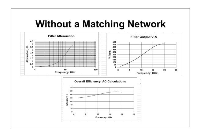
With no matching network we cannot lose any power there, but this leaves the filter with an improper termination. The result is a resonant circuit causing almost 4db peaking. In terms of V-A in the load near the upper end of the band, power goes from ~180 to over 450V-A. The efficiency graph looks like a patent should be applied for. The reason for this is recirculating currents in our newly formed resonant circuit.
