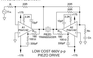
Two PA41/42 amplifiers operated as a bridge driver for a piezo transducer provides a low cost 660 volt total drive capability. The  $R_{\scriptscriptstyle N}\,C_{\scriptscriptstyle N}$  network serves to raise the apparent gain of A2 at high frequencies. If  $R_{\scriptscriptstyle N}$  is set equal to R the amplifiers can be compensated identically and will have matching bandwidths.
