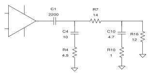
FIGURE 7. A SAMPLE COMPLEX LOAD (PARASITICS NOT SHOWN)
