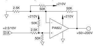
FIGURE 17. SINGLE SUPPLY OPERATION:  $V_{\text{CM}}$ CONSIDERATIONS
