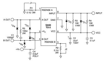
\* D<sub>1</sub> and D<sub>2</sub> – Input protection, high speed such as IN4148. D<sub>3</sub> through D<sub>6</sub> – Flyback protection, high speed (<200nS). Solder as close to SA50 as possible.
