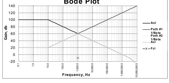
As frequency increases, impedance of the inductor increases and being inside the feedback loop it is causing closed loop gain to increase. Another way to view it: The amplifier's job is to drive constant current but as frequency goes up it needs more voltage to maintain that constant current, so voltage gain is increasing with frequency.
