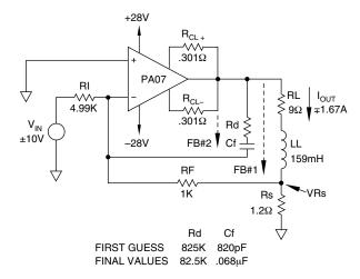
FIGURE 16. V-I CIRCUIT AND STABILITY
