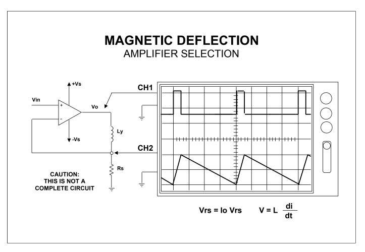
An amplifier selected for magnetic deflection must have an adequate slew rate and voltage rating to slew the current in the yoke fast enough.
