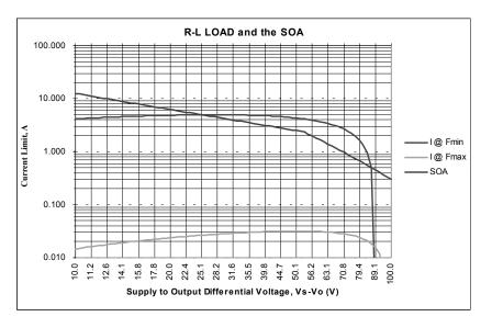
Can a 125W, 10A device drive this 5A load? It's a large coil (250mH and  $4.5\Omega$ ) and the frequency is only 5Hz. If efficiency were only 50%, delivering this 112VA to the load should be OK, shouldn't it? No. And no.
