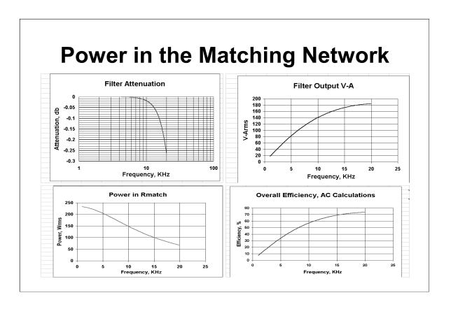
While the conjugate matching network performs almost like magic in terms of forcing the attenuation graph to near text book shape, there is a cost involved. This cost is slight when the load is mostly resistive but power dissipated in this network approaches power delivered to the load as the load approaches pure reactance.
