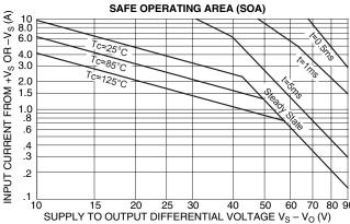
The SOA curves combine the effect of all limits for this Power Op Amp. For a given application, the direction and magnitude of the output current should be calculated or measured and checked against the SOA curves. This is simple for resistive loads but more complex for reactive and EMF generating loads. The following guidelines may save extensive analytical efforts.
