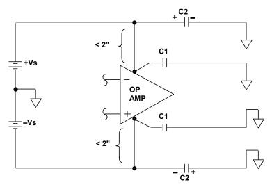
C1 = 0.1 to  $1\mu$ F, Ceramic C2 =  $10\mu$ F/Amp out (peak), Electrolytic
