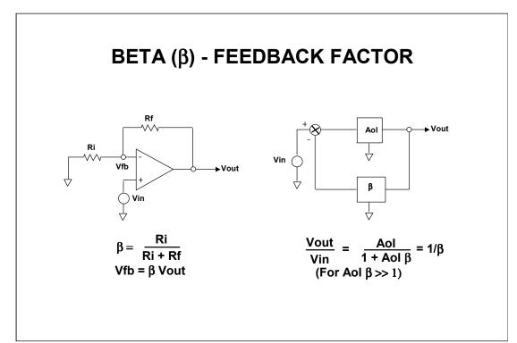
Control theory is applicable to closing the loop around a power op amp. The block diagram above in the right consists of a circle with an X, which represents a voltage differencing circuit. The rectangle with AoI represents the amplifier open loop gain. The rectangle with the  $\beta$  represents the feedback network. The value of  $\beta$  is defined to be the fraction of the output voltage that is fed back to the input. Therefore,  $\beta$  can range from 0 (no feedback) to 1 (100% feedback).
