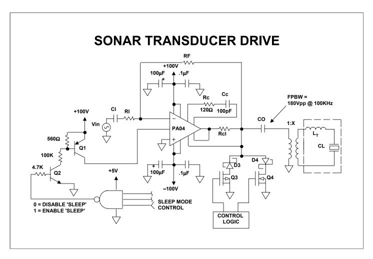
High current drive capability and wide power bandwidth make the PA04 ideally suited for sonar drive applications.
