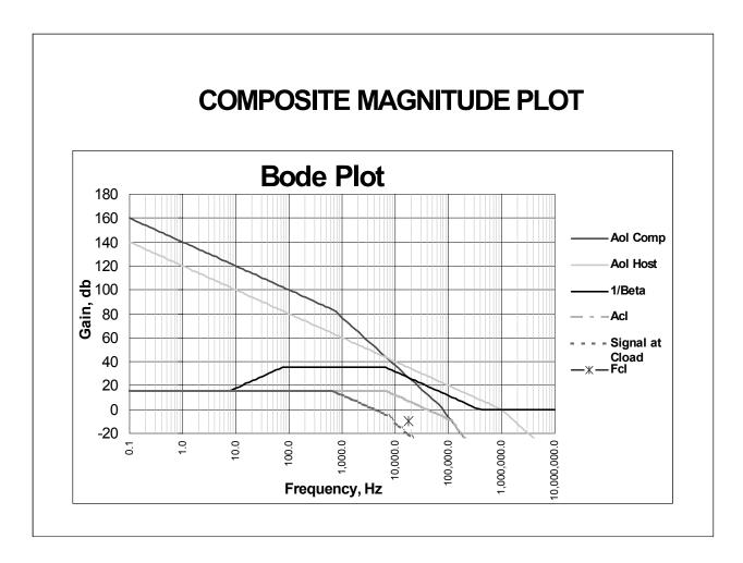
Now that the power stage is stable we add its closed loop gain to the open loop gain of the host amplifier. Note that it is the poles of the power stage rather than the host producing the -40db per decade slope in the area of interest. A roll off capacitor gives us required slope for good intersection rate and noise gain allows good placement of the actual intersection.
