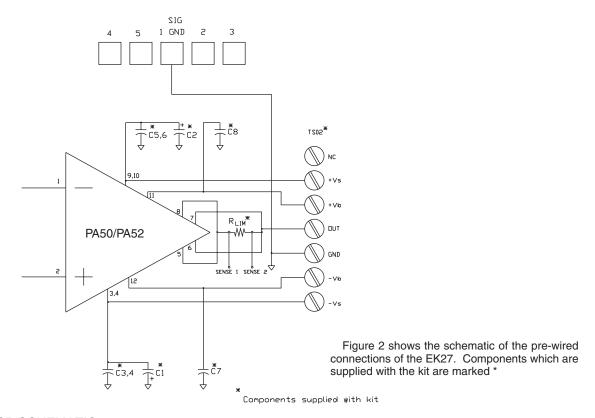
FIGURE 2. PCB SCHEMATIC.
