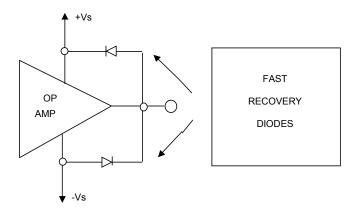
NOTE: SUPPLIES MUST BE ABLE TO ABSORB TRANSIENT ENERGY, i.e.: LOW IMPEDANCE
