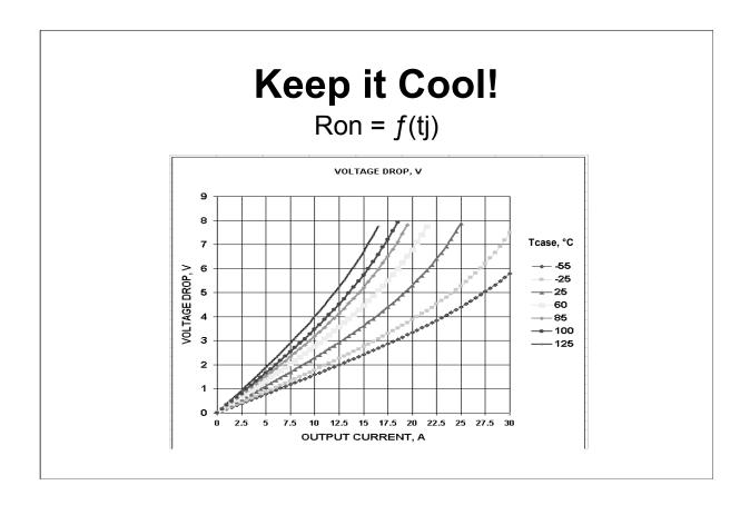
The "on" resistance of a power MOSFET increases a little over two times as junction temperature rises from +25°C to +150°C. This means a larger heatsink increases both output capability and efficiency. If there's good news to this story it's the non-linearity of the curve: The first few degrees we lower temperatures buys the most. Here's a way to approach the problem.
