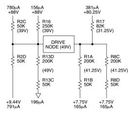
FIGURE 4. CURRENT BALANCING OF THE DRIVE NODE
