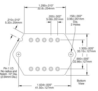
PIN DIAMETER: 1.47/1.57mm or .058/.062" PIN LENGTH: 11.43/12.70mm or .450/.500"
