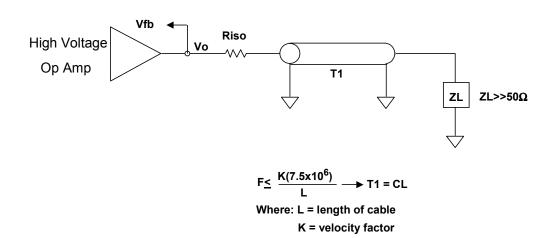
High voltage power op amps often drive their loads via coax and these are often not terminated in the characteristic impedance of the cable. This means the coax is primarily adding capacitive loading to the op amp unless the cable length is at least one-fortieth of wavelength at the frequency of interest.
