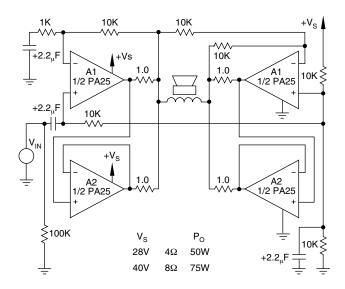
FIGURE 7. SINGLE SUPPLY PARALLEL BRIDGE
