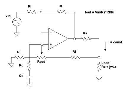
Inductive loads cause stability trouble with current source applications. Because current lags voltage in an inductor, current feedback is delayed and thus decreases the phase margin of the current amplifier. Consequently, ringing or oscillation occurs. This following procedure shows a proper compensation technique for inductive loads.
