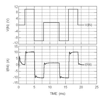
After power up settling, the first 3msec pulse accelerates the motor toward the work piece; the second 3msec pulse decelerates the motor; a constant pressure is held for 60msec (time was compressed in this plot); the last two pulses move the motor back to home position; and at t=150msec the cycle is repeated.
