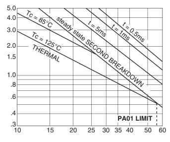
The SOA curves combine the effect of these limits. For a given application, the direction and magnitude of the output current should be calculated or measured and checked against the SOA curves. This is simple for resistive loads but more complex for reactive and EMF generating loads.
