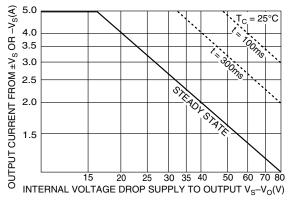
The SOA curves combine the effect of these limits and allow for internal thermal delays. For a given application, the direction and magnitude of the output current should be calculated or measured and checked against the SOA curves. This is simple for resistive loads but more complex for reactive and EMF generating loads. The following guidelines may save extensive analytical efforts:
