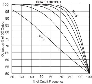
FIGURE 5. REDUCED POWER AS FSIGNAL APPROACHES FC
