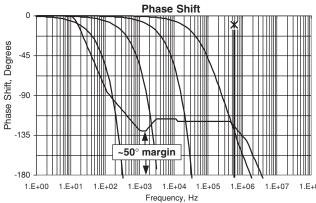
FIGURE 14. COMBINING NOISE GAIN WITH A ROLL OFF CAPACITOR
