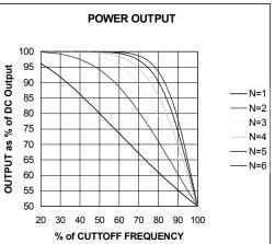
Designing the cutoff frequency at twice the actual maximum signal frequency is a very common technique to obtain a flatter response in the portion of the pass band actually used. You can see that in cases where amplitude flatness is critical, higher order filters and a wider ratio between actual signal frequency and Fc both help.
