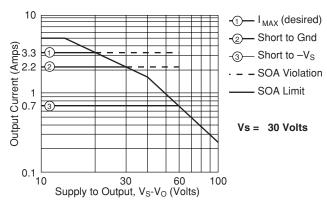
FIGURE 6. CURRENT LIMIT FAULT PROTECTION
