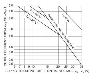
The amplifier can handle any EMF generating or reactive load and short circuits to the supply rails or shorts to common if the current limits are set as follows at  $T_{\rm c}=85^{\circ}{\rm C}$ .
