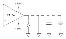
FIGURE 3. DIFFICULT LOADS OR POSSIBLE FAULT CONDITIONS
