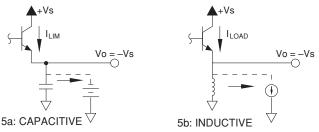
FIGURE 5. TRANSIENT STRESS WITH REACTIVE LOADS
