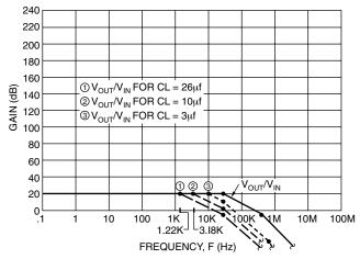
FIGURE 20.  $V_{OUT}/V_{IN}$  FOR VARIOUS CL
