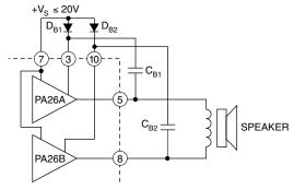
FIGURE 3. SIMPLE BOOTSTRAPPING IMPROVES POSITIVE OUTPUT SWING. CONNECT PINS 3 AND 10 TO  $V_{\rm S}$  IF NOT USED. TYPICAL CURRENTS ARE 12mA EACH.
