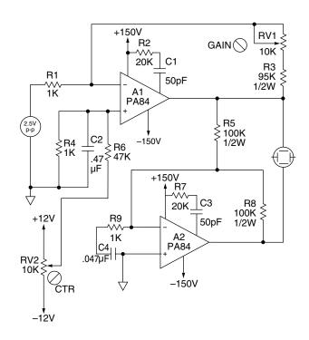
FIGURE 3. ELECTROSTATIC DEFLECTION AMPLIFIER
