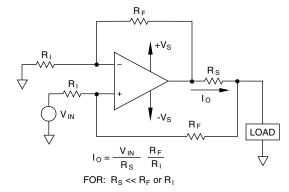
FIGURE 7. VCCS FOR A GROUNDED LOAD
