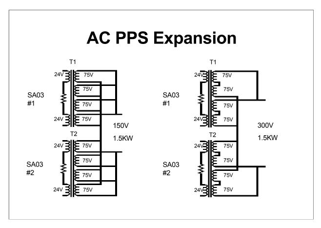
Yes, there really was a reason for four secondaries in the previous slide. With a slave module importing the AC signal from the master the two amplifiers will be in phase at the signal frequency even though they may not be in phase at the switching frequency.
