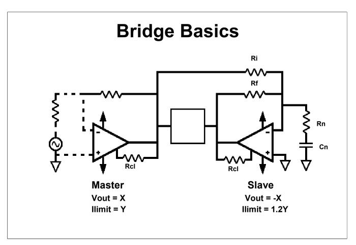
The master amplifier in the bridge may be configured in any manner suitable for a single version of the particular model. Set gain of the slave for ½ the total required to drive the load. The slave provides the other half of the gain by inverting the output of the master and driving the opposite terminal of the load. Dual supply operation is the easiest but asymmetric or single supply versions are also common.
