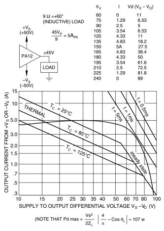
FIGURE 5. TYPICAL LOAD LINE CALCULATIONS
