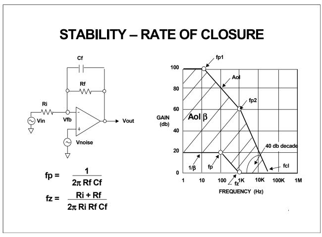
The example above shows a typical single pole op amp configuration in the inverting gain configuration. Notice the additional Vnoise voltage source shown at the + input of the op amp. This is shown to aid in conceptually viewing the  $1/\beta$  plot.
