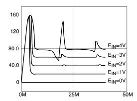
FIGURE 5A. SMOOTHING CAPACITOR C1=1000  $\mu$ F
