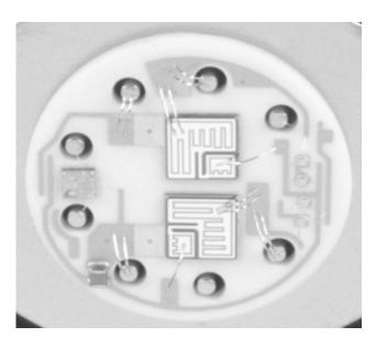
With a minimum transistor count and no resistors, the class "C" amplifiers enjoy a roomy layout. The power transistors are soldered to silver thick film conductors. Small signal devices are epoxied and wire bonded to gold thick film conductors. Wire bonds are 1 mil and 5 mil diameter. The white ceramic substrate is beryllium oxide (BeO) which spreads the heat over a wide area before it travels through the steel header. The substrate is also solder attached.
