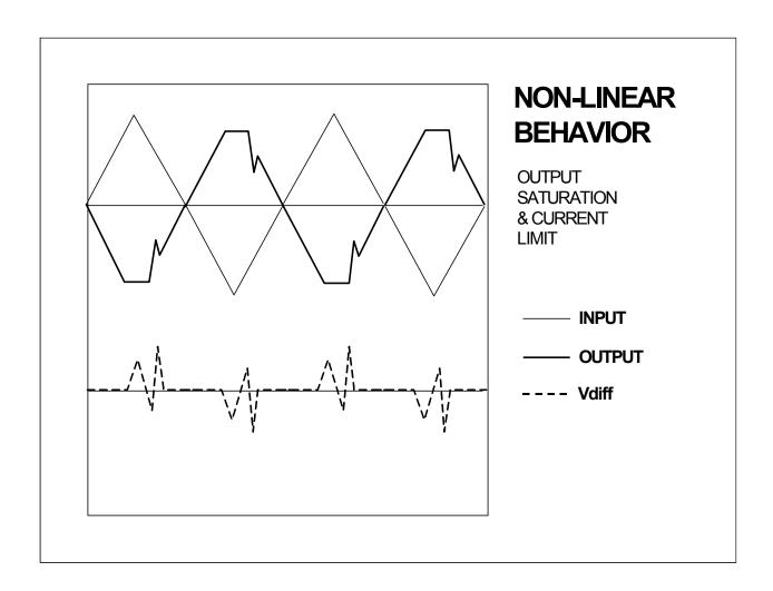
Output saturation and current limit exhibit similar behavior — clipping on the amplifier output. This clipping produces differential input voltages.
