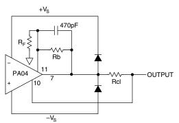
FIGURE 3. FOLDOVER CURRENT LIMITING CIRCUIT
