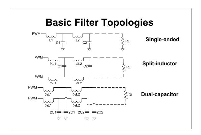
No matter what topology is used, a first order filter would use only L1, a second order adds C1, a third order adds L2, and so on. Each pole of the filter adds 20db/decade to the slope or roll-off of the filter.
