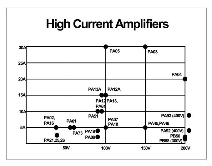
From the plastic packaged PA26 for USD\$4.95 @1K to the PA03 for USD\$525 @1, Apex covers a very wide spectrum of multiple ampere models. Typical power response ranges from 13KHz to 3.5MHz.
