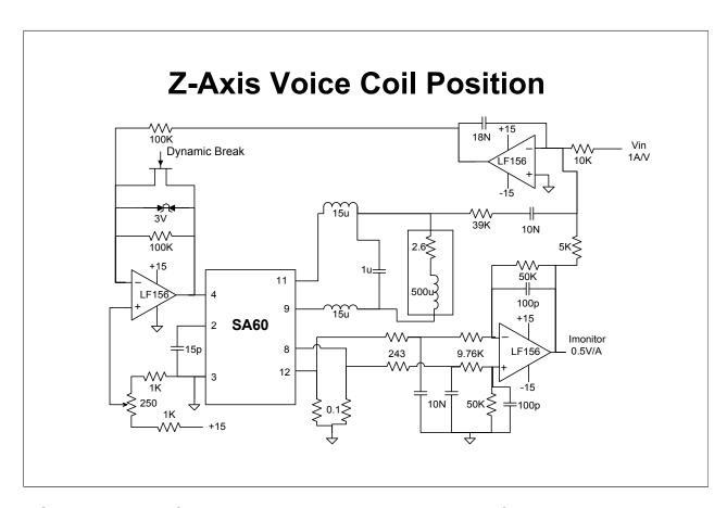
Slower versions of this machine used a PA12 linear op amp for Z-axis control. Even though currents were lower and motor impedance was higher, an exotic custom heat sink had to be designed to fit the small physical location of the amplifier. It was clear that this generation of the machine required higher efficiency in the drive circuit. The SA60 provides this and being programmed to switch at about 220KHz, it provides adequate bandwidth for the high speed servo loop.
