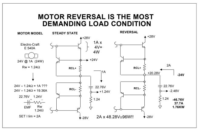
A DC motor driven at 24V with 1A steady state current flow and a winding resistance specified at  $1.24\Omega$  can be modeled as a resistor in series with an EMF. In this example since the 1A drops 1.24V across the  $1.24\Omega$ , the remaining 22.76V is back EMF.
