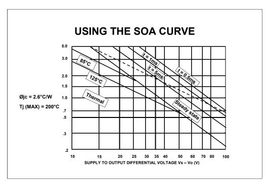
Safe operating area curves show the limitations on the power handling capability of power op amps. There are three basic limitations.
