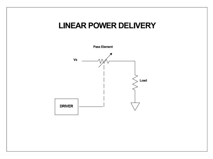
As power levels increase the task of designing variable drives increases dramatically. While the array of linear components available with sufficient voltage and current ratings for high power drives is impressive, a project can become unmanageable when calculation of internal power dissipation reveals the extent of cooling hardware required. Often the 20A drive requires multiple 20A semiconductors mounted on massive heatsinks, usually employs noisy fans and sometimes liquid cooling is mandated.
