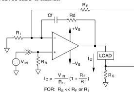
FIGURE 2. VCCS FOR FLOATING LOAD; INCREASED GAIN CONFIGURATION
