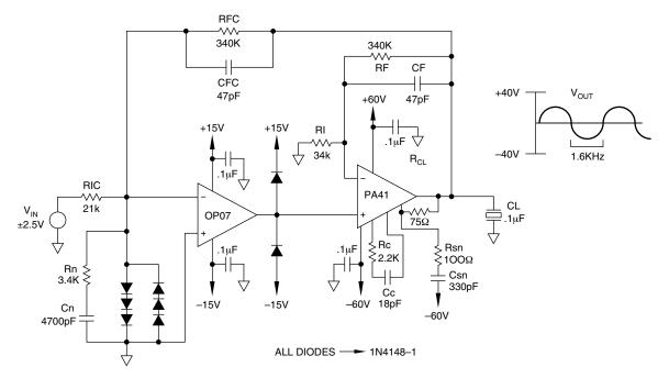
FIGURE 33. PA41 COMPOSITE PIEZO TRANSDUCER DRIVE
