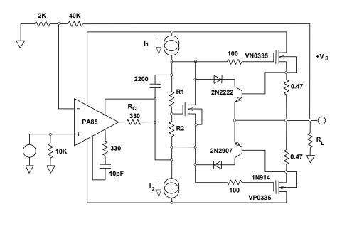
The class C circuit was able use a simplified version of this slide with no attempt to establish class A/B bias in the MOSFET output stage. In that circuit with no bias, the typical MOSFET threshold of 3V means the op amp must swing 6V during the crossover transition while the final output does not move. The additional circuitry used here will lower distortion and is increasingly important as frequency goes up. Distortion improvements better than an order of magnitude have been achieved.
