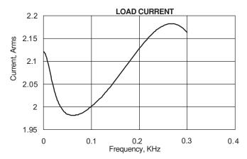
FIGURE 30. CURRENT OUTPUT WITH THE MODIFIED MATCHING NETWORK
