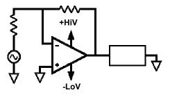
There's something very appealing about a circuit with only two gain setting resistors. Many times there is already a low voltage supply in the system just waiting to be used. This supply need only provide quiescent current of the op amp unless the op amp swings negative or in the case of reactive loads where current and voltage are not in phase.
