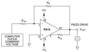
MICROMOVEMENT: LOW POWER, PIEZOELECTRIC POSITIONING
