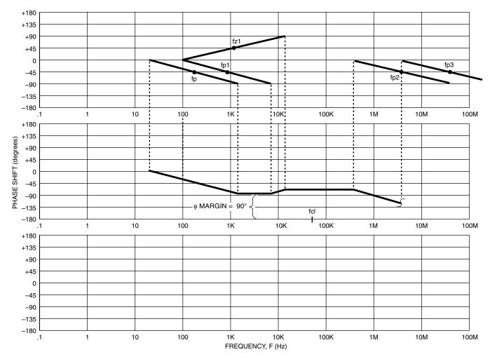
FIGURE 15. OPEN LOOP PHASE PLOT FOR STABILITY CURVE (2) (w/R<sub>ISO</sub>)
