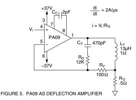
If 50% of the total transition time is allowed for slewing and settling,  $2\mu s$  will remain to change the yoke current with full voltage applied to the coil. Voltage requirements are calculated as follows:
