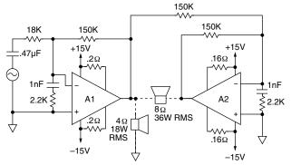
FIGURE 6. DOUBLING POWER WITH A BRIDGE
