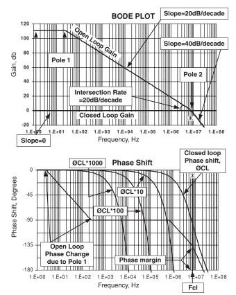
FIGURE 3. UNITY GAIN STABLE AMPLIFIER CURVES
