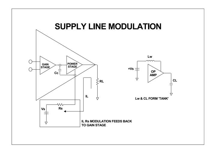
Supply loops are another source of oscillation. In one form of power supply related oscillations the load current flowing through supply source resistance and parasitic trace resistance modulates the supply voltage seen at the power supply pin of the op amp. This signal voltage is then coupled back into a gain stage via the compensation capacitor which is usually referred to one of the supply lines as an AC ground.
