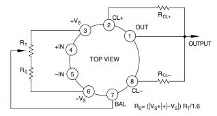
NOTE: Input offset voltage trim optional.  $R_T = 10K\Omega$  MAX 8-pin TO-3 package
