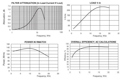
FIGURE 18. RESULTS OF A MODIFIED MATCHING NETWORK
