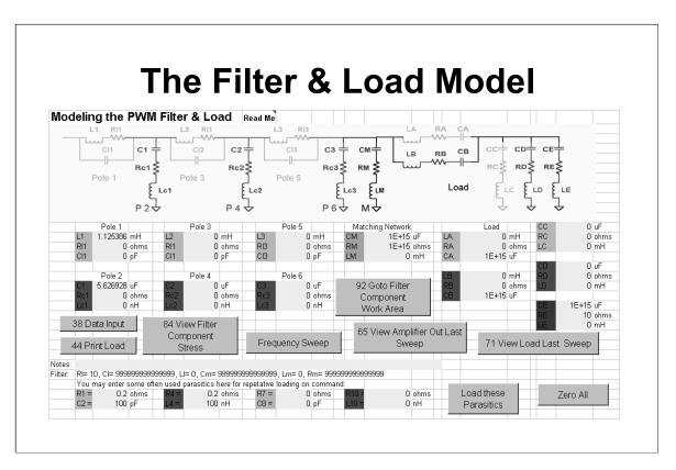
Pressing one of the "Load All Data" buttons on the PWM Filter sheet transfers your application to the PWM Power sheet. Ideal component values are loaded automatically for all six pole elements, the matching network and on the far right, the load we specified earlier. Extra components in the load modeling area provide more flexibility. As the math (and execution time) would be a significantly larger burden for any other topology, Power Design only analyzes single-ended filters.
