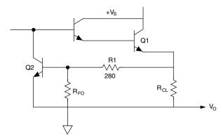
FIGURE 4. BASIC FOLDOVER CURRENT LIMIT CIRCUIT
