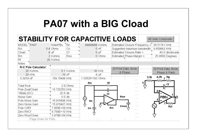
This basic circuit will demonstrate how each of the capacitive load compensation techniques can work independently to solve the large C load stability problem.
