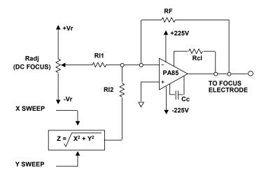
RAPID CORRECTION OF FOCUS FOR HIGH RESOLUTION DISPLAYS
