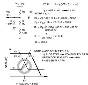
FIGURE 23. FEEDBACK NO. 2 (FB #2) FINAL VALUE CALCULATIONS
