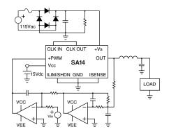
AC/DC POWER CONVERSION: PWM CREATES TRANSFORMERLESS CONVERSION
