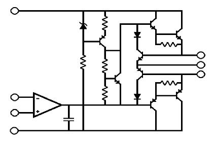
The class "AB" output keeps some current flowing in the output transistors at all times to minimize crossover distortion. This area is still the largest contributor to total harmonic distortion but the "dead" band is gone.
