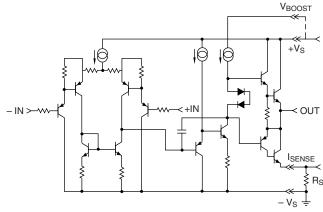
FIGURE 2. PA26 EQUIVALENT SCHEMATIC (ONE CHANNEL)
