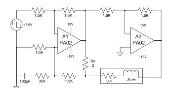
FIGURE 6. CURRENT-OUT BRIDGE DRIVE
