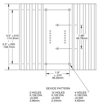
Standard Commercial **Extrusion Tolerances Apply** Material: Aluminum Alloy Finish: Black Anodize Thermal Resistance: ≈ .96°C/W Approximate Weight: 19.8 oz
