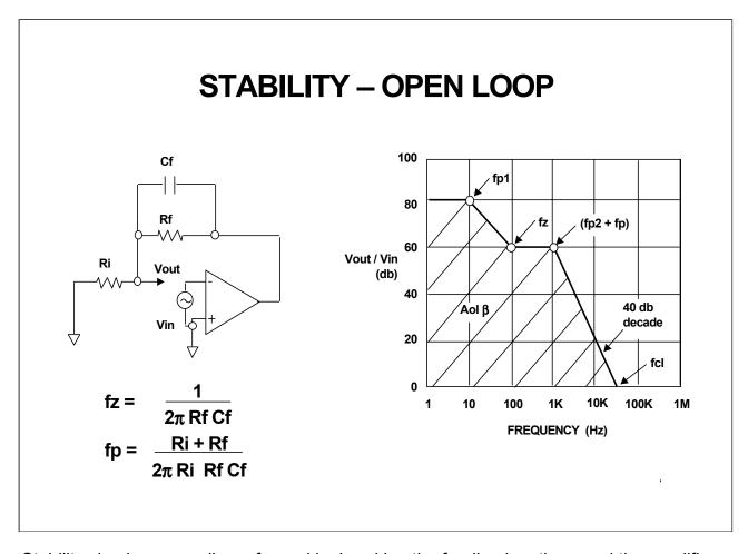
Stability checks are easily performed by breaking the feedback path around the amplifier and plotting the open loop magnitude and phase response. This open loop stability check has the first order criteria that the slope of the magnitude plot as it crosses 0 dB must be 20 dB per decade for guaranteed stability.
