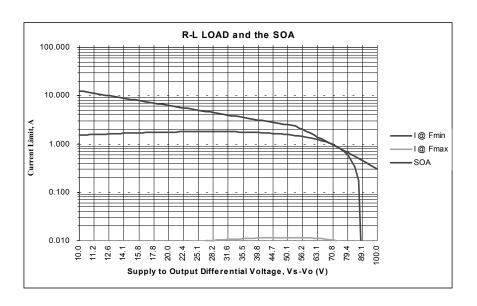
Reducing the load requirements all the way to  $25\Omega$  produces a load line not in violation of the second breakdown curve and power dissipation in the amplifier is down to a manageable 82W.
