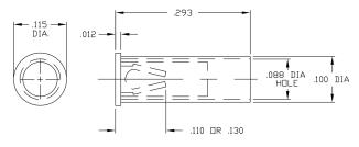
SOLDER MOUNT IN .102 MIN. MOUNTING HOLE T□L = ±.003
