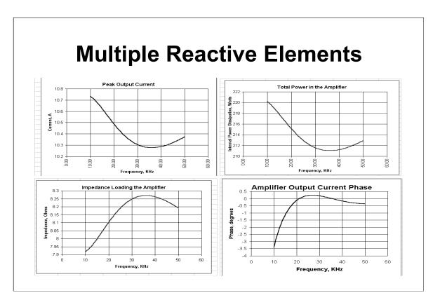
Any time an application has more than one reactive element, peak values of voltage, current, phase shift and power dissipation may not be at the minimum or maximum frequencies. It would be a good idea to run a frequency sweep to locate worst case operating points.
