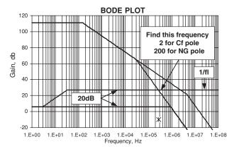
FIGURE 13. SETTING UP THE INITIAL NOISE GAIN CURVE
