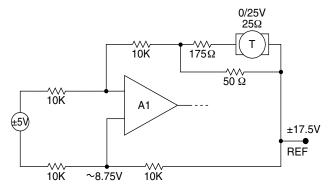
FIGURE 2. HIGH OUTPUT TACHOMETER
