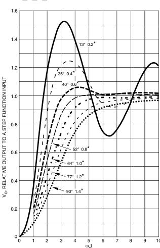
\* OPEN LOOP PHASE MARGIN AND DAMPING FACTOR
