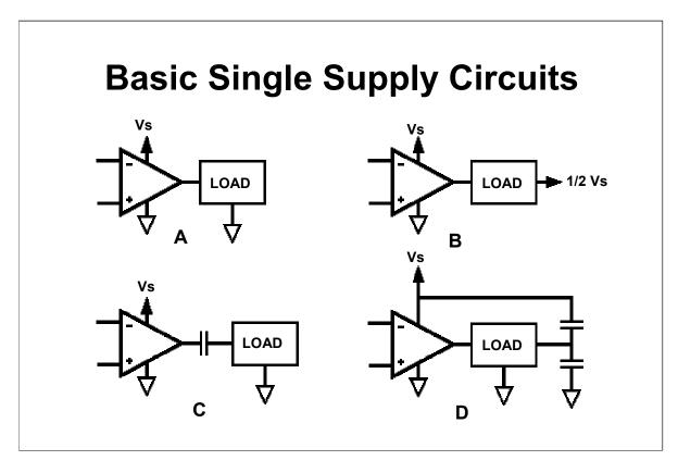
Circuit A is only suitable for unipolar and non-zero inclusive drives. These type applications might include Programmable Power Supply (PPS), heater controls and unidirectional speed controls.
