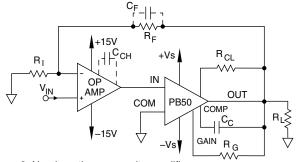
Figure 2. Non-inverting composite amplifier.
