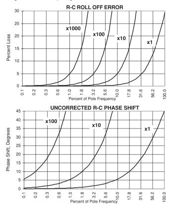
FIGURE 15. R-C ROLL OFF AMPLITUDE ERROR AND UNCORRECTED PHASE SHIFT
