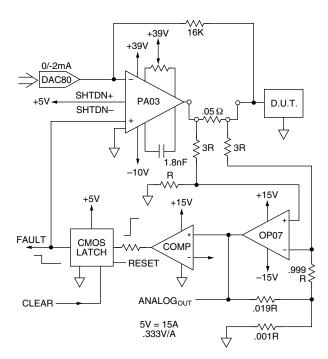
FIGURE 5. HI-POWER PROGRAMMABLE POWER SUPPLY APPLICATION
