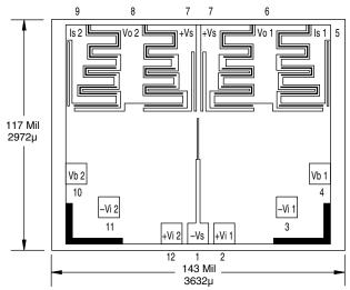
Thickness: 18 Mil ±2 Mil Backside: Ni Ag 20,000 Å (min) Bond pad: 10 Mil sq (254µ) **NOTE:** Backside at -V<sub>s</sub> potential.
