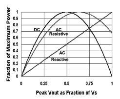
Cranking the volume or the output up to maximum is <u>not</u> necessarily the worst case internal power dissipation for a linear output stage. We saw earlier that under DC and resistive load conditions, 50% of supply voltage was worst case.
