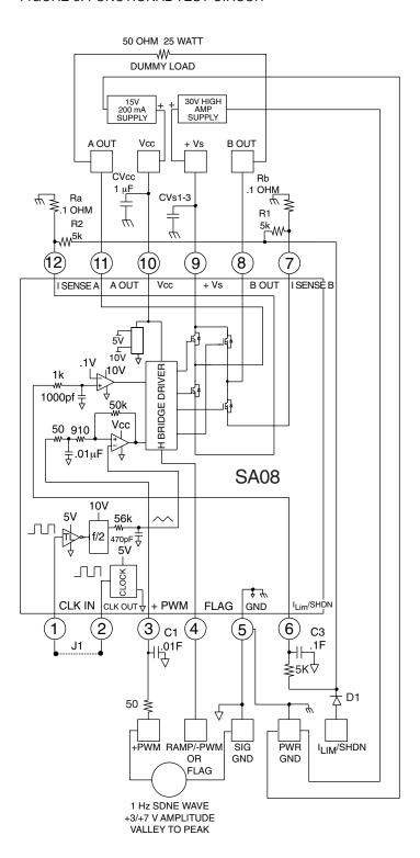
The schematic of Figure 3 can be used to verify the functionality of your amplifier and help you gain a familiarity with proper operation. At either A Out or B Out, with respect to ground, you should observe a square wave approximately 30 V in amplitude with a fixed frequency and duty cycle that varies from approximately 0 to 100% at a rate of 1 Hz. The current limit is set to 2 amps.
