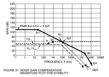
$$fp2 = \frac{1}{2\pi \text{ Ro CL}} = \frac{1}{2\pi 100 159 \text{nF}} = 10 \text{KHz}$$
