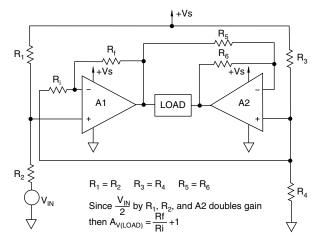
FIGURE 5. MODIFIED SINGLE-SUPPLY BRIDGE FOR IMPROVED SUPPLY REJECTION
