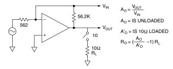
FIGURE 2. OUTPUT IMPEDANCE MEASUREMENT CIRCUIT
