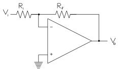
FIGURE 2. BASIC INVERTING CONFIGURATION.
