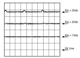
FIGURE 6B. ADDING A 10,000 μF IN PARALLEL WITH C1 LOWERS OUTPUT RIPPLE, ESPECIALLY AT HIGH CURRENT LEVELS.
