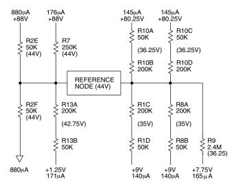
FIGURE 3. CURRENT BALANCING OF THE REFERENCE NODE
