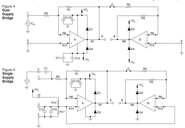
equal to R3 to configure the slave amplifier as a unity gain inverter.
