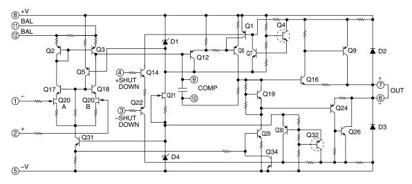
FIGURE 8. PA03 EQUIVALENT SCHEMATIC
