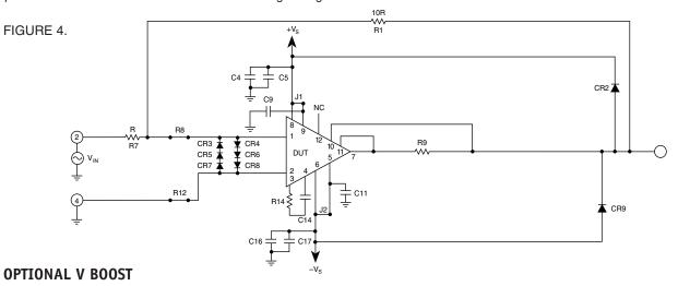
One of many inexpensive ways to acquire V boost for the PA04 has been included as an option on this evaluation kit. The addition of these parts not only increases swing, but also extends the
