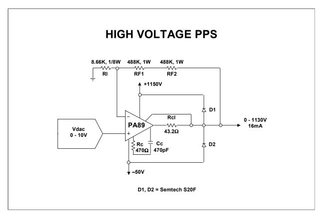
This high voltage programmable power supply utilizes the full voltage capability of the PA89. It uses asymmetrical power supplies to eliminate the necessity for biasing up the front end input DAC voltage to comply with common mode voltage requirements of the PA89, as well as providing adequate voltage headroom at the output so it can swing down to zero.
