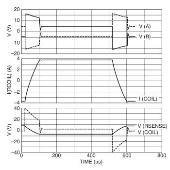
FIGURE 5. MAGNETIC DEFLECTION VOLTAGE AND CURRENT WAVEFORMS
