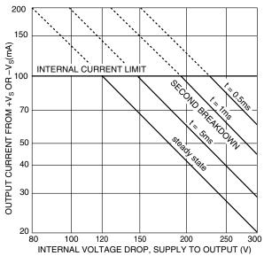
The SOA curves combine the effect of these limits. For a given application, the direction and magnitude of the output current should be calculated or measured and checked against the SOA curves. This is simple for resistive loads but more complex for reactive and EMF generating loads. However, the following guidelines may save extensive analytical efforts:
