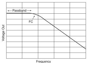
FIGURE 1. LOW PASS FILTER RESPONSE
