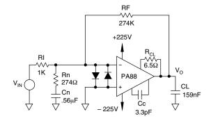
FIGURE 30. NOISE GAIN COMPENSATION FOR CL
