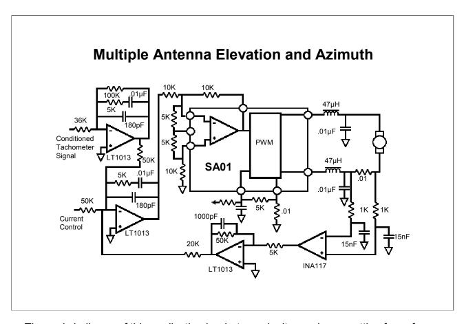
The real challenge of this application is what you don't see above; putting four of these circuits on one PC card. The motors have a minimum inductance of 300µH and have current ratings from 4.6A to 16.7A on 48V. The drive circuit needs to be universal with a current drive and a velocity loop to be used under some circumstances.
