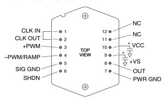
Case tied to pin 5. Allow no current in case. Bypassing of supplies is required. Package is Apex MO-127/40S. See Outline Dimensions/Packages in Apex data book.
