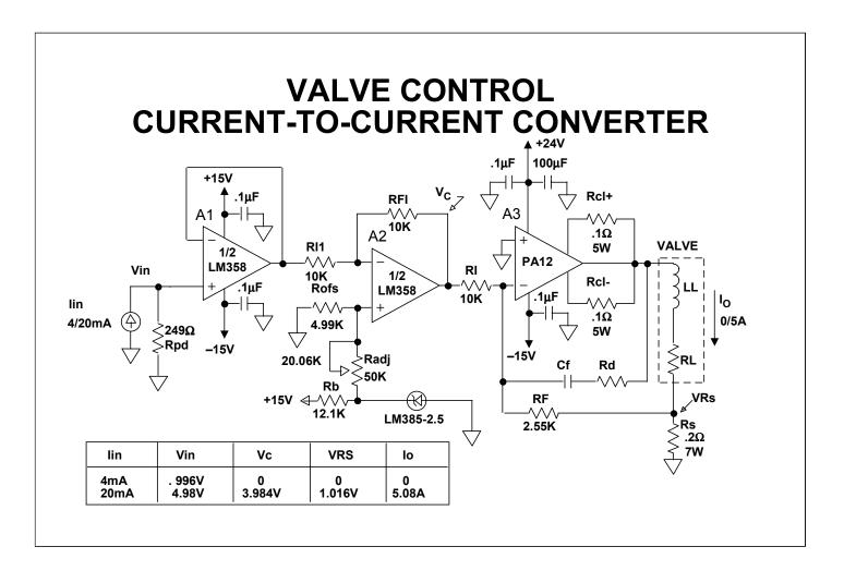
This circuit provides a Current-to-Current converter function through translation of a 4-20mA current transmitter to 0-5A output for linear control of a valve.
