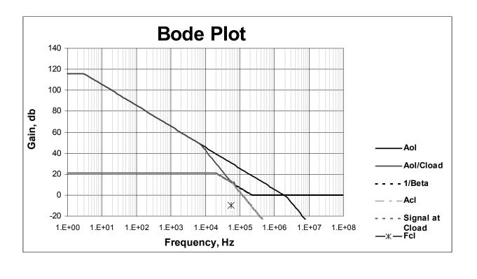
In any composite amplifier, make sure the power output stage is stable first. Any of the techniques we learned earlier can be used.
