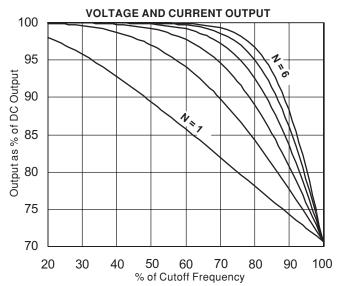
FIGURE 4. REDUCED V & I AS FSIGNAL APPROACHES Fc
