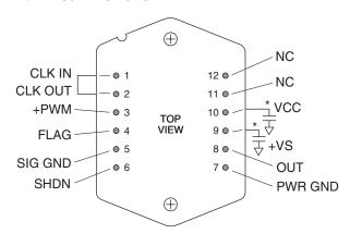
Case tied to pin 5. Allow no current in case. Bypassing of supplies is required. Package is Apex MO–127 (STD). See Outline Dimensions/Packages in Apex data book.
