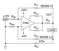
FIGURE 1. PROGRAMMABLE POWER SUPPLY WITH REMOTE SENSING
