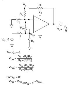
FIGURE 3. SINGLE SUPPLY NON-INVERTING CONFIGURATION
