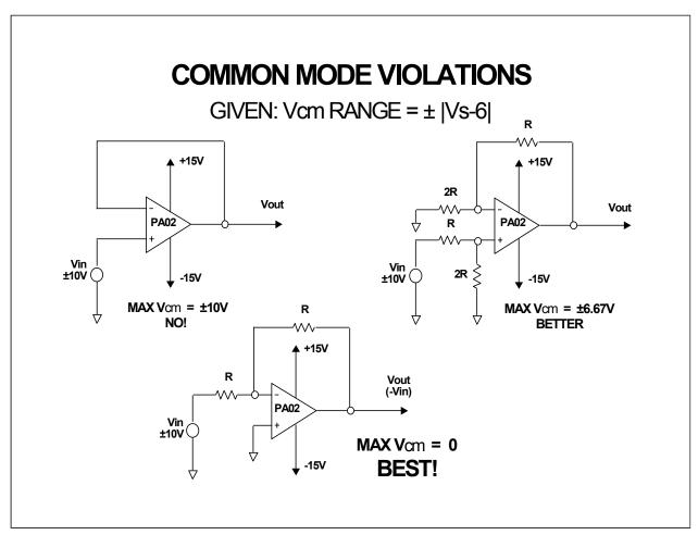
In an inverting configuration, the op amps non-inverting terminal is usually tied to ground, making the inverting terminal a "virtual ground." This results in zero common mode voltage: a desirable benefit. However, operating the amplifier in a non-inverting mode results in the common mode voltage being equal to the voltage at the non-inverting terminal.
