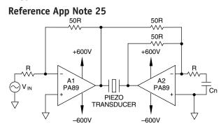
SINGLE AXIS MICRO-POSITIONING, ±1150V
