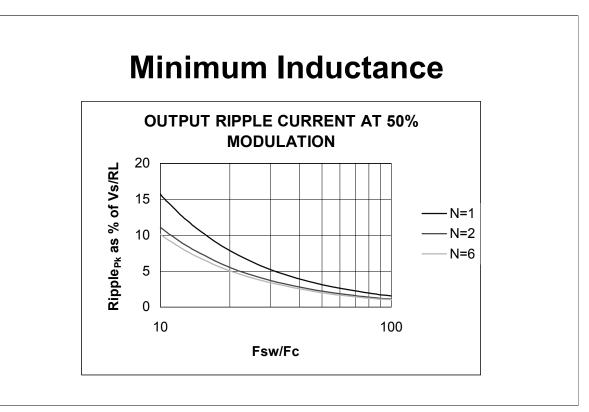
Application Note 30 admonishes us to make sure the PWM amplifier is driving enough inductance to keep ripple current at the switching frequency to a reasonable level. When designing filters according to Application Note 32, this concern becomes part of the filter design.
