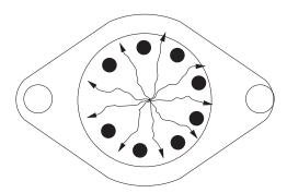
FIGURE 15. MAIN HEAT FLOW PATH: 8-PIN TO 3 PACKAGE
