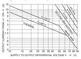
The SOA curves combine the effect of all limits for this Power Op Amp. For a given application, the direction and magnitude of the output current should be calculated or measured and checked against the SOA curves. This is simple for resistive loads but more complex for reactive and EMF generating loads. However, the following guidelines may save extensive analytical efforts.
