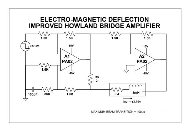
A1 is a Howland Current Pump, A2 provides a gain of -1 to drive the opposite terminal of the coil. A first glance, it might appear the choice of  $2\Omega$  for the sense resistor is quite large because the peak voltage drop across it is 7.5V, or half the supply voltage.
