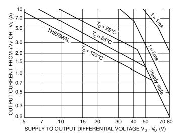
The SOA curves combine the effect of of all limits for this Power Op Amp. For a given application, the direction and magnitude of the output current should be calculated or measured and checked against the SOA curves. This is simple for resistive loads but more complex for reactive and EMF generating loads. The following guidelines may save extensive analytical efforts.
