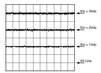
FIGURE 6C. WORKS WITH A WIDE RANGE OF LOADS. WITH R1 OPEN, HIGH FREQUENCY RIPPLE IS HIGHER BECAUSE OUTPUT LC FILTER IS UN-TERMINATED.
