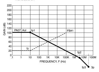
FIGURE 17. AoI AND FB # 1 - MAGNITUDE PLOT FOR STABILITY
