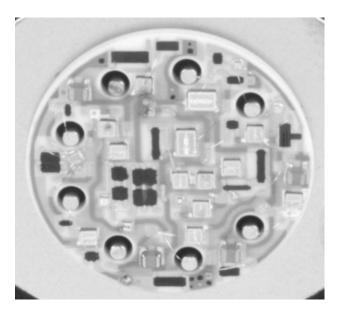
Real estate is at quite a premium with the complex designs. The only new thing added here is the blue glass layer covering most of the conductor traces. It has a two fold purpose: It is a bonding aid and an electrical insulator. This model happens to be a 450 volt part.
