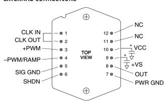
Case tied to pin 5. Allow no current in case. Bypassing of supplies is required. Package is Apex MO-127 (STD). See Outline Dimensions/Packages in Apex data book.
