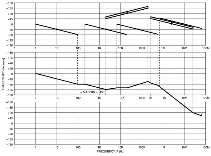
FIGURE 19. COMPOSITE OPEN LOOP PHASE PLOT FOR STABILITY
