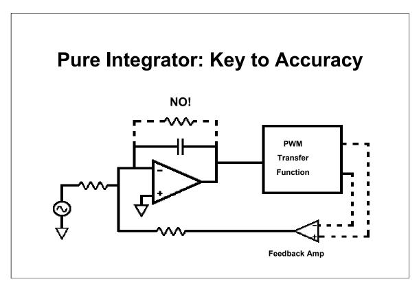
Lets go back to some basic op amp theory for a moment: The open loop gain (the voltage ratio of the output pin to difference of the input pins) of an op amp is extremely high (100db is 100K:1). This means the input pin voltage above is approaching zero. If there is no DC feedback and no current in or out of the input pin, then current through the two resistors must be equal. The PWM output is accurately scaled to the input signal.
