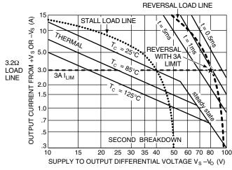
FIGURE 1. EXAMPLE OF MOTOR DRIVE LOAD LINE ANALYSIS
