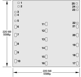
Thickness: 11 Mil (280µ) Backside: Silicon (no back metal) Small Bond pads: 5 Mil sq (127µ) Al
