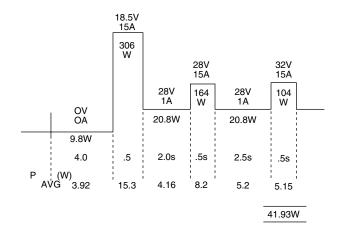
FIGURE 6. PROGRAMMABLE POWER SUPPLY INTERNAL POWER DISSIPATION
