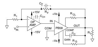
Figure 2. Non-inverting composite amplifier.
