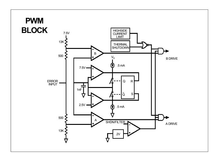
The oscillator portion of the PWM controller consists of two comparators, two switched current sources charging the timing capacitor and a flip-flop. When voltage on the timing capacitor reaches 7.5V, the upper comparator resets the flip-flop which opens the upper current source and connects the lower one. When the timing capacitor voltage reaches 2.5V, the lower comparator sets the flip-flop to start the next cycle.
