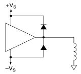
FIGURE 1. PROTECTION, INDUCTIVE LOAD
