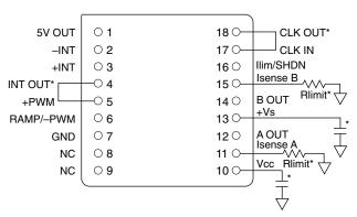
Case tied to Pin 7. Allow no current in case. Bypassing of supplies is required. Package is Apex DIP6. See Outline Dimensions/Packages. If +PWM > RAMP then A OUT > B OUT.
