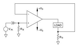
FIGURE 1A. BASIC VCCS FOR FLOATING LOAD
