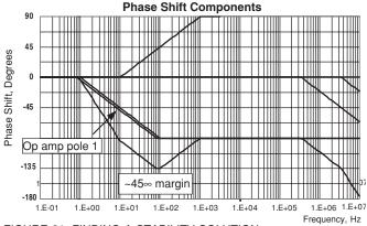
FIGURE 21. FINDING A STABILITY SOLUTION
