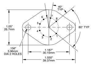
PIN CIRCLE DIAMETER .500" OR 12.7mm PIN DIAMETER .090" or 2.29mm
