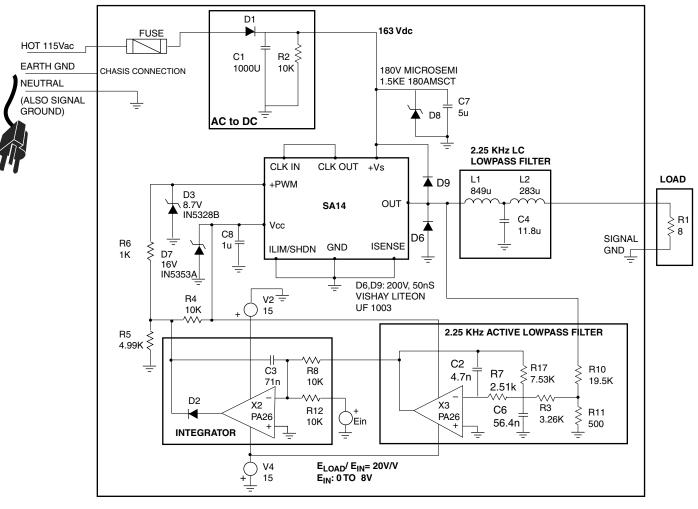
FIGURE 3. DETAILED TRANSFORMERLESS AC TO DC CIRCUIT DIAGRAM.
