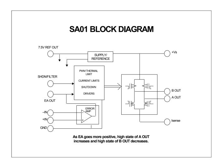
PWM circuits are taking the same general course of development traveled by op amps and many other electronic functions. Concepts were brought to life using discrete components and were followed by modules, hybrids and then monolithics. The first hybrid on the scene in PWM technology is the SA01 from Apex. The amplifier contains all the functions needed to implement a wide variety of control circuits.
