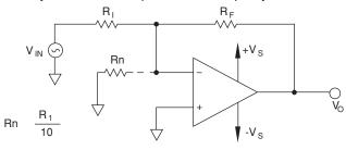
FIGURE 20. LOOP CHECK CIRCUIT
