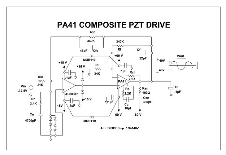
This circuit is included as an example in Power Design.xls. It is different from most power op amps in that current limit from positive side to negative side does not match well at all.
