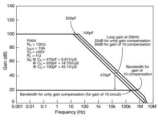
FIGURE 2. THE SMALL SIGNAL RESPONSE FOR THE PA04
