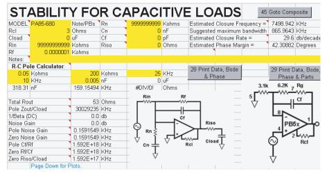
FIGURE 2. DATA ENTRY FOR CLOAD ANALYSIS
