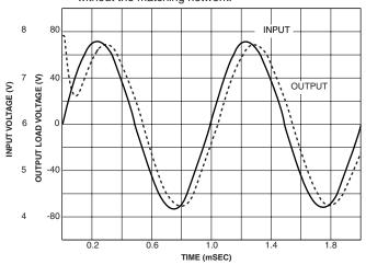
FIGURE 7. Ignoring the feedback circuitry of X3 abd X4, a 1-kHz, 3.5V p-p sine wave with offset at Vin produces a 120V p-p sine wave across the load.
