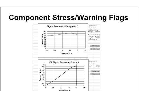
Power Design calculates voltage and current stress levels on L1 and L2, plus C1 and C2 for all designs. Resonance of these filters can produce voltages and currents larger than the load levels. Button 84 will place the first graph on the screen, then scroll up and to the right to view other graphs. The currents shown here can be used directly for all filter topologies. If L1 is actually two inductors, half the voltage shown will be across each individual inductor.
