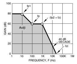
FIGURE 14. STABILITY- OPEN LOOP
