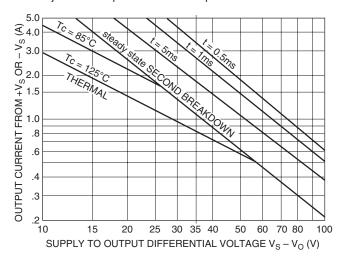
The SOA curves combine the effect of these limits. For a given application, the direction and magnitude of the output current should be calculated or measured and checked against the SOA curves. This is simple for resistive loads but more complex for reactive and EMF generating loads.
