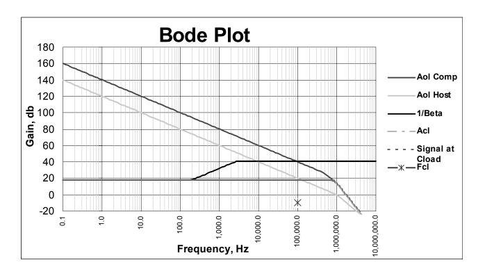
This circuit is not battling capacitive loading or inductance in the feedback path and each part of the composite would be stable on its own but the composite open loop gain reaches a slope of -60db per dacade before crossing 0db.
