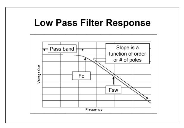
PWM filters are normally low pass configuration. These exhibit low attenuation to the frequency spectrum from 0 Hertz to the frequency of cutoff (Fc). This low attenuation region is called the pass band. Beyond the Fc, attenuation increases at a rate determined by the filter type and the numbers of poles (order).
