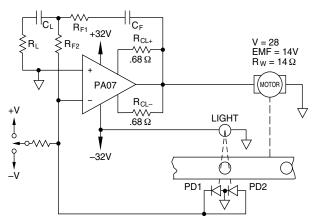
Negates optoelectronic instabilities Lead network minimizes overshoot SEQUENTIAL POSITION CONTROL
