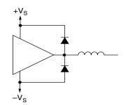
FIGURE 2. PROTECTION, INDUCTIVE LOAD
