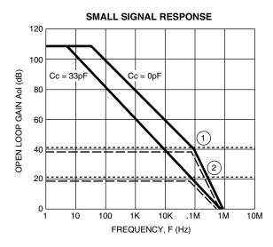
FIGURE 12. EXTERNAL PHASE COMPENSATION
