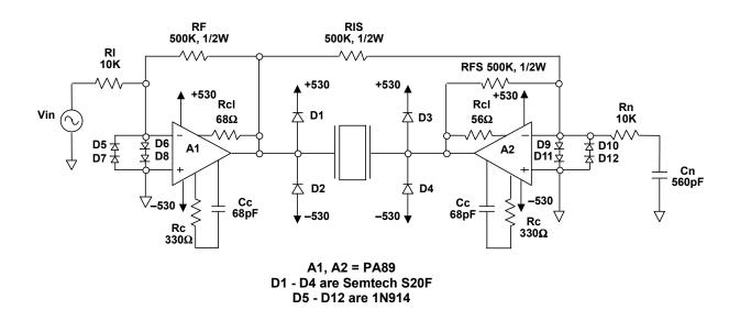
Piezo users appear to never have enough voltage. As soon as it was introduced the PA89 found its way into bridge circuits to drive piezos at +/1100V and beyond.
