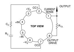
C<sub>C</sub> IS NPO RATED FOR FULL SUPPLY VOLTAGE.
