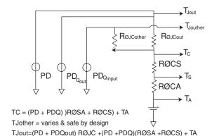
FIGURE 13. MORE ACCURATE THERMO-ELECTRIC MODEL
