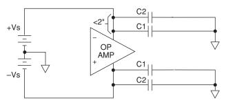
C1 = .1 to .1∝F, Ceramic, High Frequency Bypass C2 = 10∝F/Amp out (peak), Electrolytic/Tantalum, Low Frequency Bypass
