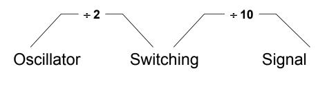
The alternate ramp generator illustrated the relationship between oscillator and switching frequencies. Some PWM data sheets (such as the SA01) do not mention oscillator frequency because there is no divide by two circuit.
