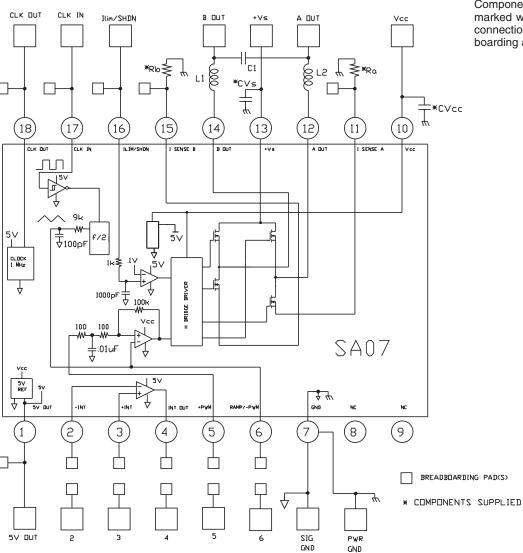
Figure 2 shows the schematic of the evaluation kit's pre-wired connections Components supplied with the kit are marked with an asterisk (\*). All other connections are made via the breadboarding areas of the circuit board.
