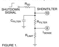
at pin 10 is referenced to pin 4 (GND). CFILTER will filter both the current limit noise spikes and the shutdown signal. Shutdown and current limit operate on each cycle of the internal switching rate. As long as the shutdown signal is high the output will be disabled.
