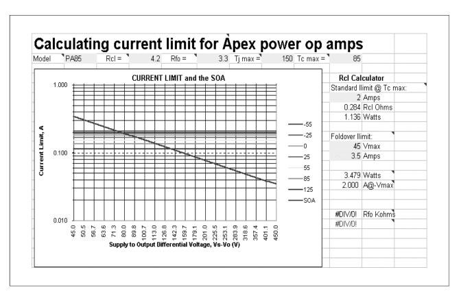
The Ilimit sheet of Power Design.xls really shows the temperature variation. It's a good thing most of us don't have to cover -55° to 125°C. Not all op amps have this slope, but the spreadsheet knows the details of each model. Also enter your limit on junction temperature.
