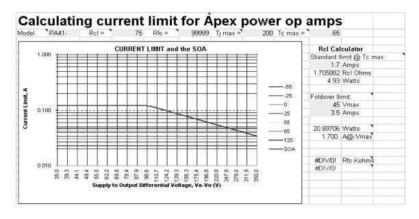
If we can assume the PA41 never gets colder than 25°C, nominal current limit is 33mA. Again, thinking about 20% tolerance, we can count on 25mA output capability.
