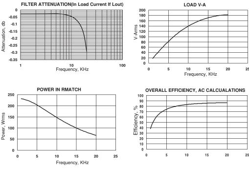
FIGURE 16. PERFORMANCE OF THE PROPERLY TERMINATED FILTER
