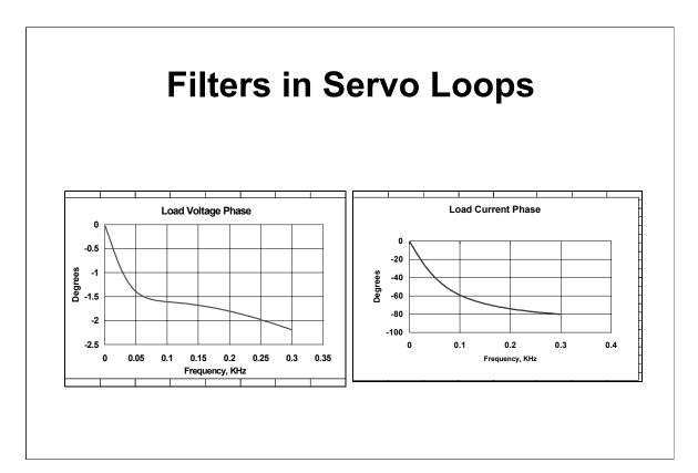
These filters are notorious for introducing large phase shifts. This is usually not a problem when feedback is taken directly at the output of the PWM amplifier. In applications such a servo loops, feedback is taken after the filter and any phase shift introduced here affects system phase margin. Power Design calculates both voltage and current phase in the load.
