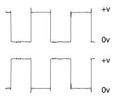
FIGURE 2. OUTPUT WAVEFORMS AT AOUT (TOP) AND BOUT (BOTTOM).
