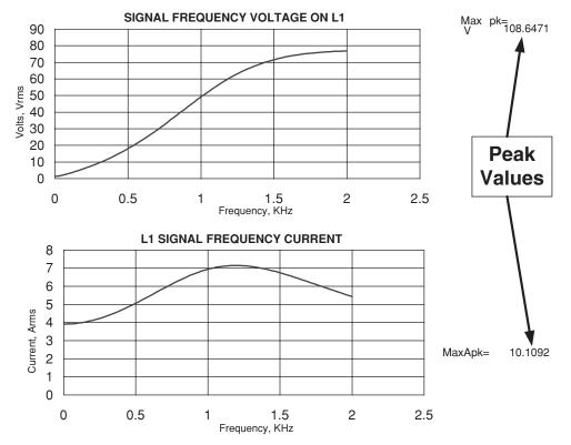
FIGURE 19. STRESS LEVELS ON L1
