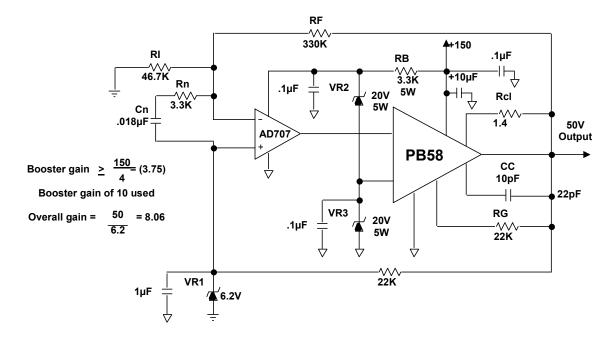
At first this may not seem to be the least costly approach to voltage regulator design. However, there is no packaged solution to regulating 150 volts down to 50 volts while being able to provide up to 500 mA (PB58 is rated up to 2A, but SOA limits us to 500 mA in this application). This regulator has both good source and good sink regulation characteristics.
