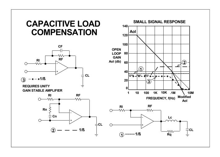
If it's necessary to use low gains with capacitive loads, or in the unlikely event they are a problem at higher gain, these techniques can help solve stability problems caused by capacitive loads.
