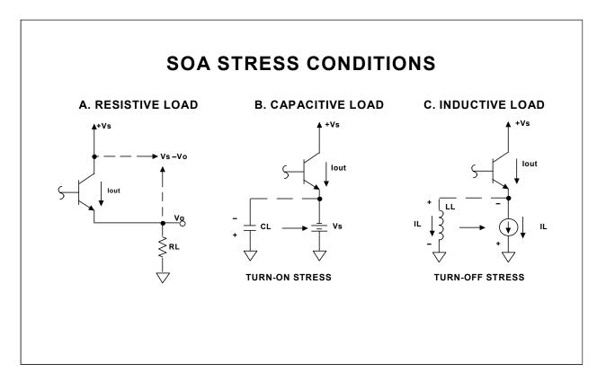
On the SOA graph, the horizontal axis,  $V_S - V_O$  does not define a supply voltage or total supply voltage or the output voltage. IT DEFINES THE VOLTAGE STRESS ACROSS THE CONDUCTING DEVICE. Thus  $V_S - V_O$  is the difference from the supply to the output across the transistor that is conducting current to the load. The vertical axis is simply the current being delivered to the load.
