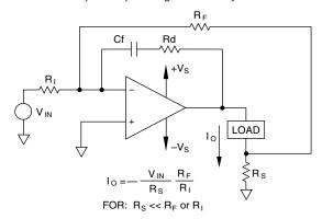
FIGURE 3. VCCS FOR FLOATING LOAD; INVERTING CONFIGURATION
