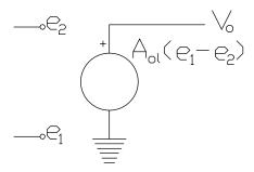
FIGURE 1. ELEMENTARY MODEL OF AN OPERATIONAL AMPLIFIER.
