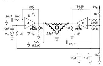
3-PHASE MOTOR DRIVE WITH 120° PHASE SHIFT
