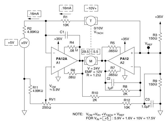
FIGURE 1. BI-DIRECTIONAL BRIDGE FOR A SINGLE SUPPLY
