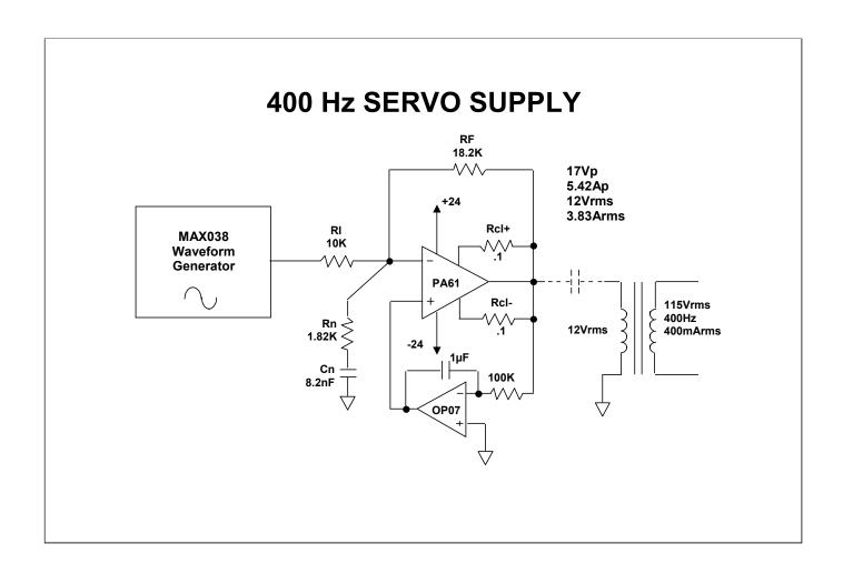
This 400Hz servo supply uses a separate oscillator to maintain oscillator stability under varying load conditions. The PA61 provides a gain of 1.8 to match the output of the industry standard 8038 waveform generator IC to the primary of a 12V to 115V step-up transformer.
