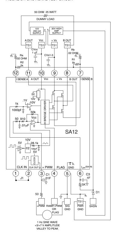
The schematic of Figure 3 can be used to verify the functionality of your amplifier and help you gain a familiarity with proper operation. At either A Out or B Out, with respect to ground, you should observe a square wave approximately 30 V in amplitude with a fixed frequency and duty cycle that varies from approximately 0 to 100% at a rate of 1 Hz. The current limit is set to 10 amps.
