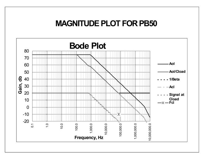
Without the isolation resistor, the modified Aol curve would have changed to -40db per decade just under 1KHz giving an unacceptable intersection rate and about 2.5° phase margin rather than 90°.
