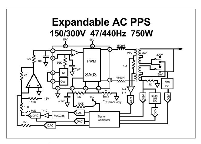
In local terms this SA03 is running open loop but overall operation is closed loop by virtue of the system computer monitoring performance and making adjustments per calibration tables and correction algorithms.
