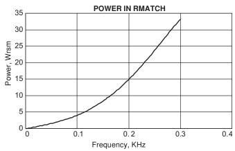
FIGURE 34. POWER DISSIPATION IN THE MODIFIED MATCHING NETWORK
