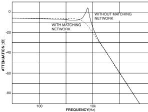
FIGURE 6. The LC filter's frequency response differs with and without the matching network.
