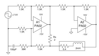
FIGURE 4. ELECTROMAGNETIC DEFLECTION AMPLIFIER
