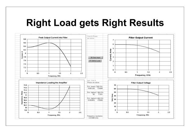
With proper termination of the filter we get a little mid-band peaking amplifier output current but the catastrophic potential of bad filter termination has gone away.
