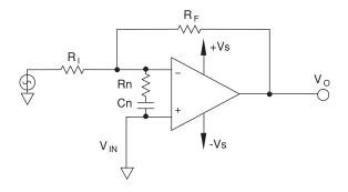
FIGURE 24. INPUT R-C NETWORK COMPENSATION
