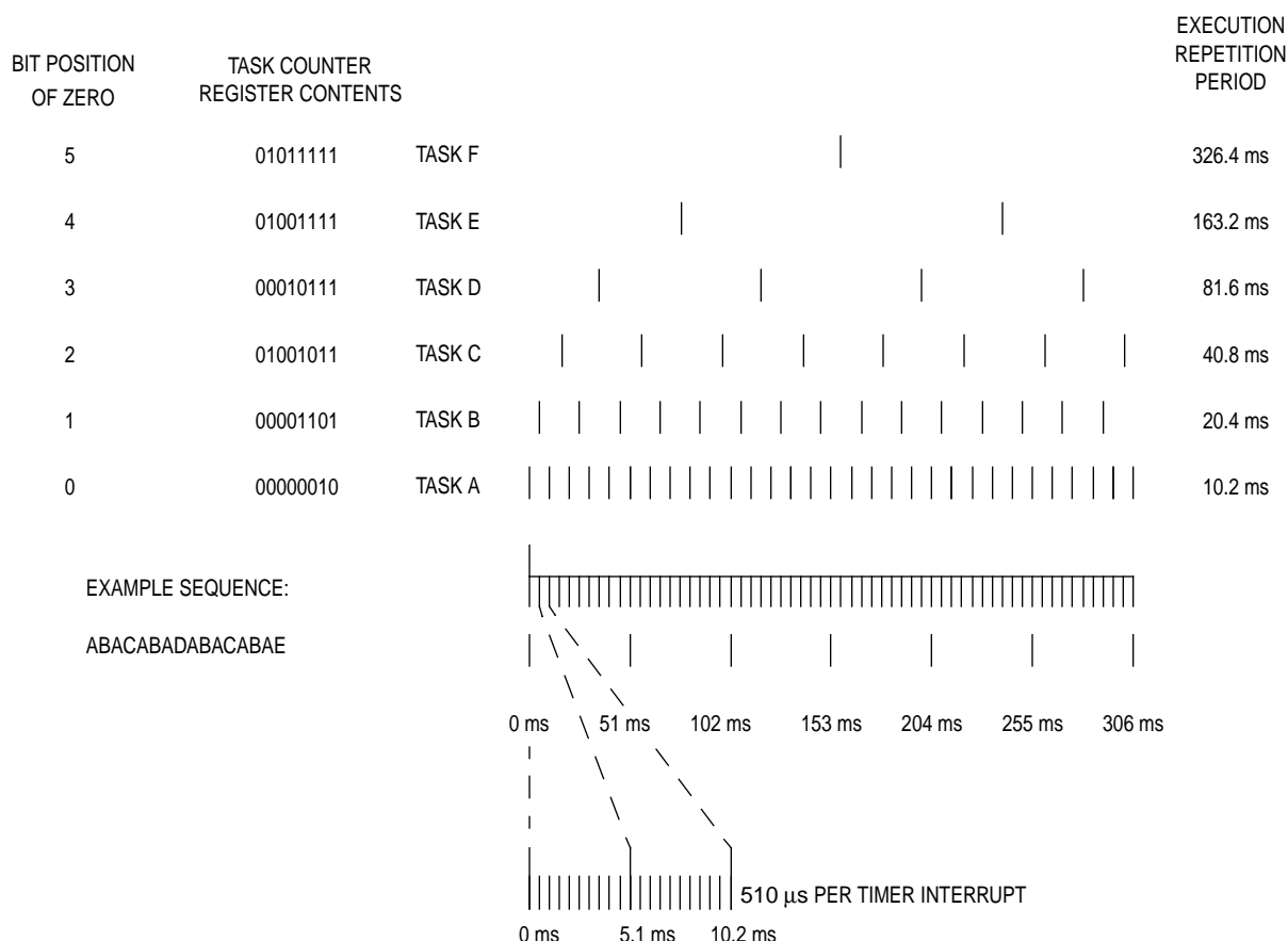
Figure 6. Example 2 — Sequence of Task Execution for Core Timer
