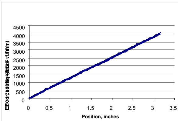
Figure 9. Final output of position sensing system after calibration
