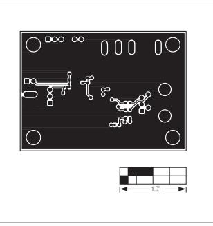
Figure 6. MAX17048X/MAX17049X EV Kits PCB Layout— Solder Side
