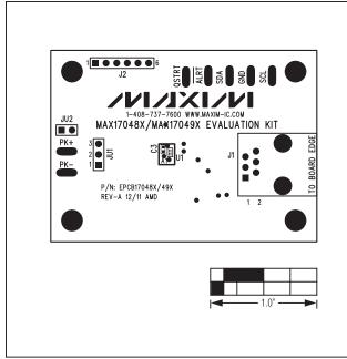
Figure 4. MAX17048X/MAX17049X EV Kits PCB Layout— Component Side
