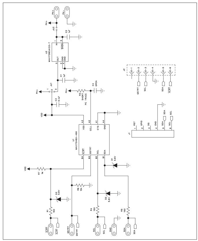
Figure 3. MAX17048X/MAX17049X EV Kits Schematic
