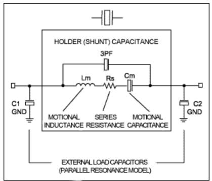
Figure 1. Generic crystal model (fundamental mode).
