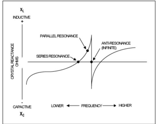
Figure 2. Crystal impedance versus frequency.
