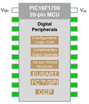
PPS enables flexible mapping of any digital peripheral to any I/O pin (green)
