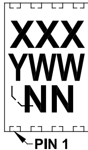
8-Lead UDFN (2x3x0.5 mm)
