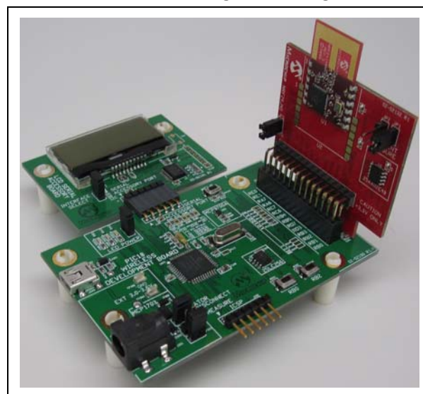
FIGURE 5: MRF24J40 MODULE ON 8-BIT WIRELESS DEVELOPMENT BOARD
