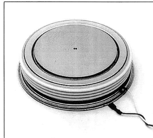
The TDS5 is a low voltage, high current, thin pack disc SCR employing a amplifying gate structure. This thin package provides greater cooling thus maximizing high current performance. The amplifying gate design allows the SCR to be reliably operated at high di/dt and dv/dt conditions in various phase control applications.
