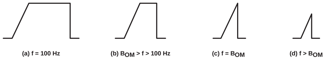
Figure 5. Full-Power-Response Output Signal
