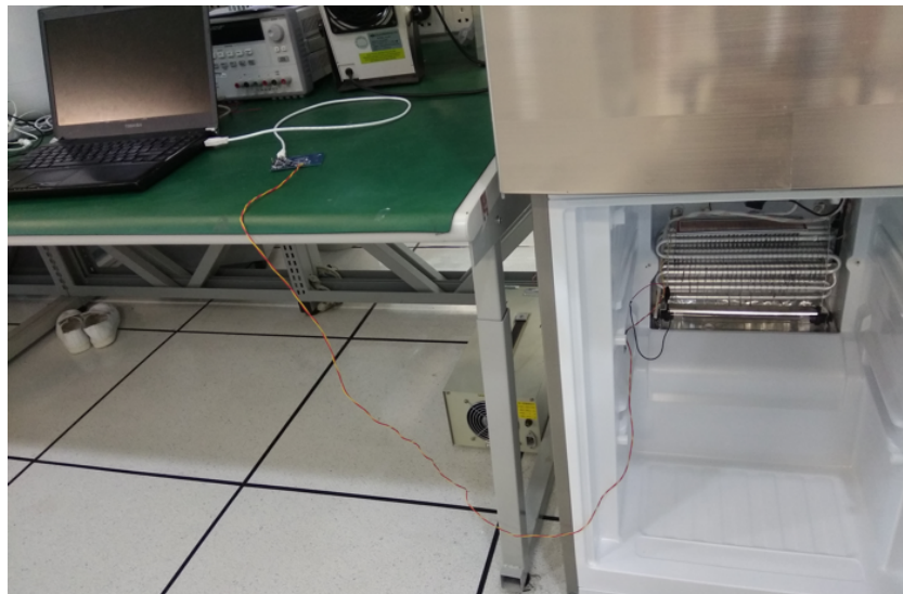
Figure 35. Long Cable Test Setup
