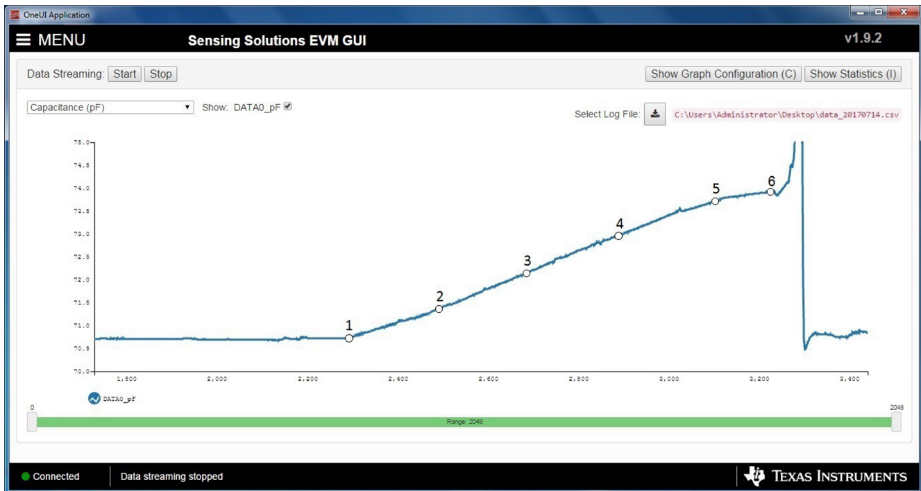
Figure 30. Sensed Capacitance During Frost Forming Process
