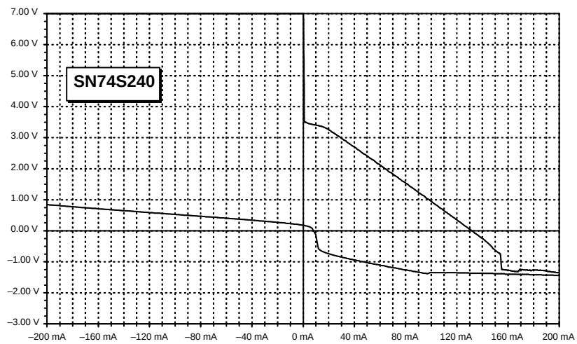
Figure 37. Output Characteristics of the SN74S240
