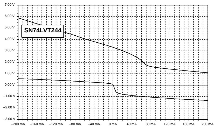
Figure 58. Output Characteristics of the SN74LVT244
