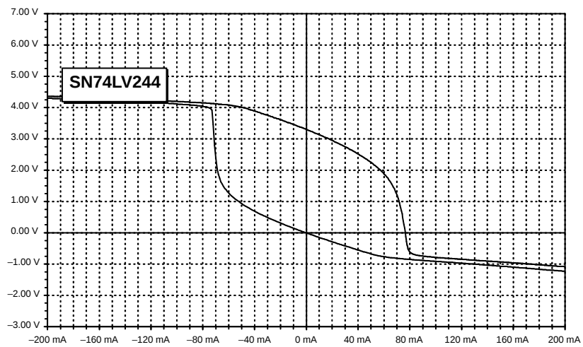
Figure 55. Output Characteristics of the SN74LV244
