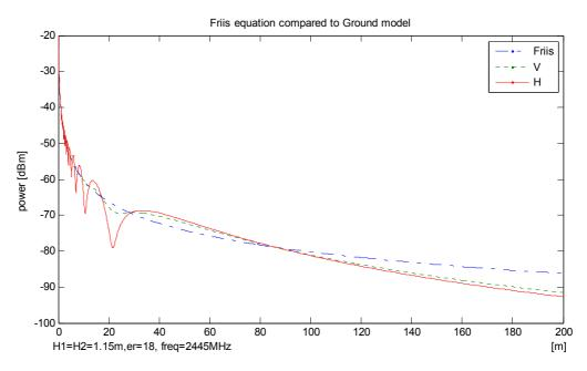
Figure 2. Difference in Transmission Loss due to Polarization
