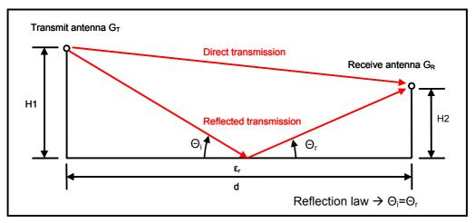
Figure 1. Transmission with Ground
