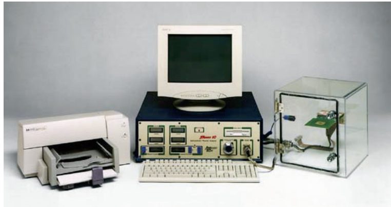
Figure 3-4: \theta_{JA} Measurement Setup
