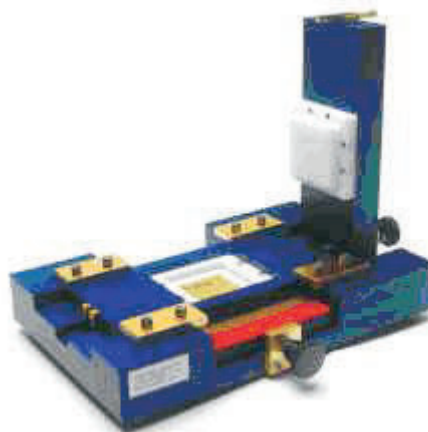
Figure 4-1: Altair BGA Fixture Used for TDR Measurement
