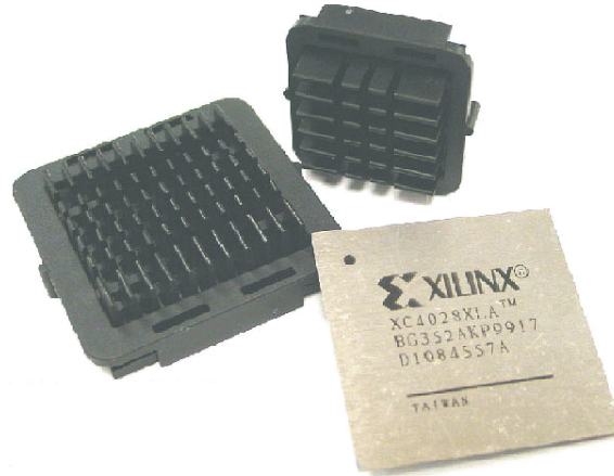
Figure 3-11: Enhanced BGA with Low Profile Retainer Type Passive Heatsinks
