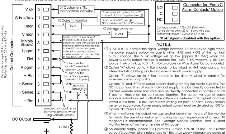
If there is any possibility of voltage from another source (another power supply, a battery, transients, etc.) being applied to the power supply's output terminals, protect the power supply by using a diode in series with either the +OUT or the -OUT.
