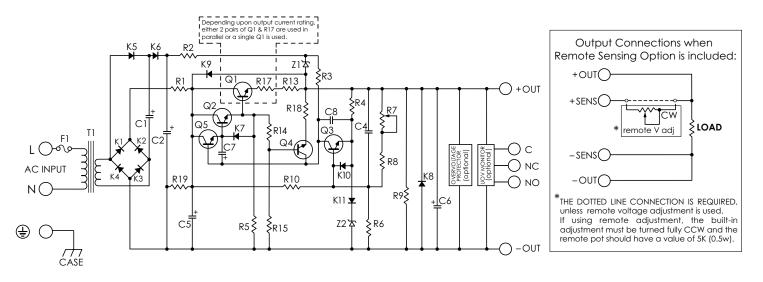
105 -125 VAC, 50-400Hz (Standard) 210-250 VAC, 50-400Hz (When model number ends in -230)
