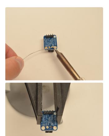
Solder again! First solder one pin by using the soldering iron to prop up the board. Then use a vice () or helper hands to hold the board in place while soldering the other pin.
