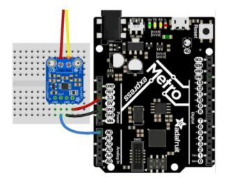
Board V+ to Metro 3.3V Board GND to Metro GND Board OUT to Metro A0 Board RED- to thermocouple red- wire Board YLW+ to thermocouple yellow+ wire
