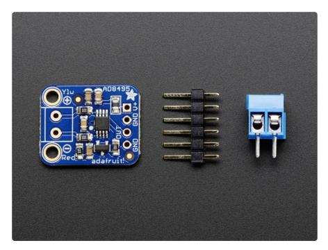
Each order comes with a 2 pin terminal block (for connecting to the thermocouple), a fully assembled PCB with the AD8495 + TLVH4311.25V precision voltage reference, and pin header (to plug into any breadboard or perfboard). Goes great with our 1m K-type thermocouple (not included) (http://adafru.it/270). Not for use with any other kind of thermocouple, K type only!
