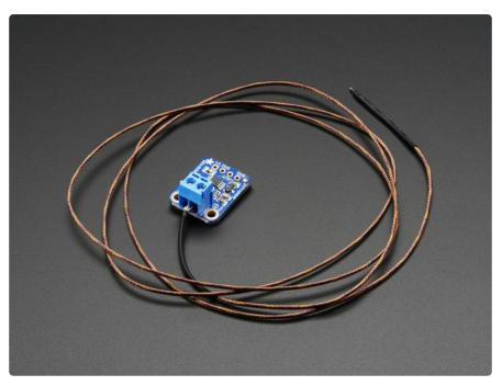
Thermocouples are very sensitive, requiring a good amplifier with a coldcompensation reference. We have a couple digital thermocouple amplifiers in the shop already from Maxim. Now we're happy to introduce an excellent analog-output amplifier. This is a very simple sensor to use, and if your microcontroller has analog input capability, you'll be ready to go really fast!
