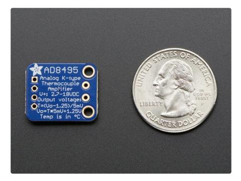
The AD8495 K-type thermocouple amplifier from Analog Devices is so easy to use, we documented the whole thing on the back of the tiny PCB. Power the board with
