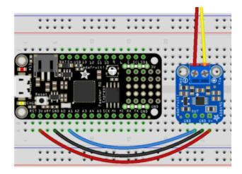
Board V+ to Feather 3V Board GND to Feather GND Board OUT to Feather A1 Board RED- to thermocouple red- wire Board YLW+ to thermocouple yellow+ wire
