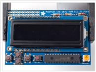
Slide the LCD over the header so that it is perfectly centered over the four holes and the silkscreen.
