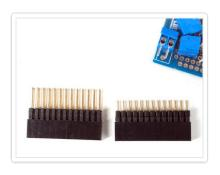
Next we will attach the header, there is a standard 'extra tall' header included in the kit. However, if you want to attach a cobbler or GertBoard, etc to the plate, you may want to opt for one of our stacking headers, they're extra long so you can plug in an IDC cable on top!
