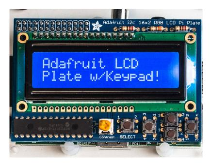
This plate is perfect for when you want to build a stand-alone project with its own user interface. The 4 directional buttons plus select button allows basic control without having to attach a bulky computer.
