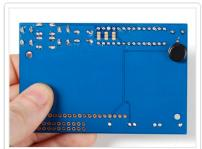
Before we solder in the header, remove the bumper from the backing and attach it on the underneath so its right over the Ethernet jack when the PCB is plugged in.
