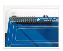
Finally, we place the LCD. Break off a piece of 18 or 16 pin header from the stick in the kit.
