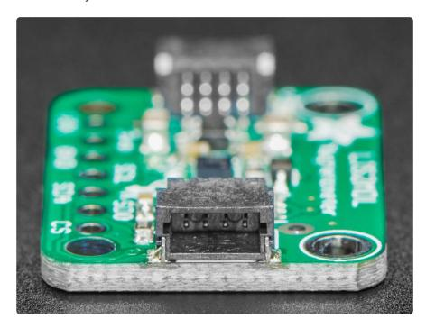
This adorable little magnetometer is quite capable but it is near-microscopic at 2mm square. To make things easier, we've put it on a breakout PCB along with support circuitry to let you use this little wonder with 3.3V (Feather/Raspberry Pi) or 5V (Arduino/ Metro 328) logic levels.
