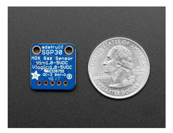
Another nice element to this sensor is the ability to set humidity compensation for better accuracy. An external humidity sensor is required and then the RH% is written over I2C to the sensor, so it can better calculate the TVOC/eCO2 values.
