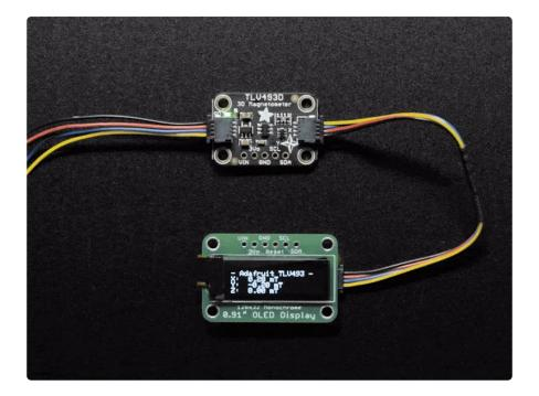
The TLV493D 3-axis magnetometer is a great little sensor for detecting magnets in 3D. (https://adafru.it/FN5) In fact, the manufacturer Infineon suggests it could be used to make a joystick! You could also use it for other cool things like detecting objects with magnets attached, like the lid of a box, or maybe a statue that unlocks your secret lair when placed on your mantle?
