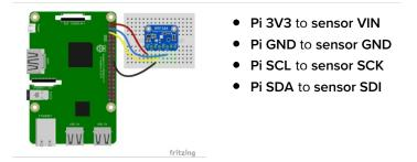
And an example on the Raspberry Pi 3 Model B wired with SPI:
