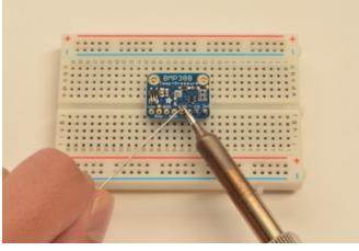
Add the breakout board: Place the breakout board over the pins so that the short pins poke through the breakout pads
