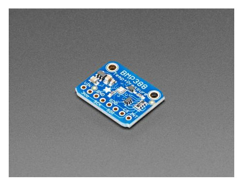
Nice sensor right? So we made it easy for you to get right into your next project. The surface-mount sensor is soldered onto a PCB and comes with a 3.3V regulator and level shifting so you can use it with a 3V or 5V logic microcontroller without worry. Check out the Arduino library to get data out in under 10 minutes! (https://adafru.it/EdV)
