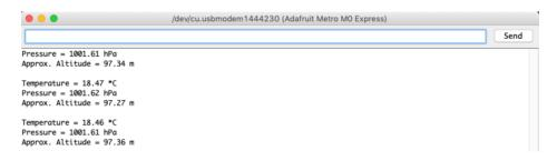
**Temperature** is calculated in degrees C, you can convert this to F by using the classic F = C \* 9/5 + 32 equation.
