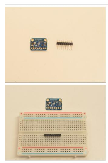
Prepare the header strip: Cut the strip to length if necessary. It will be easier to solder if you insert it into a breadboard - **long pins down**
