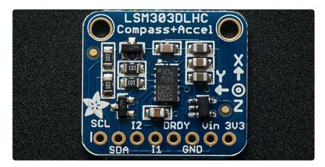
Compared to the LSM303AGR, you can see that the sensor itself (the black rectangle in the center) is physically larger. Additionally the pins are in a different order and the LSM303DLH exposes a DRDY (data ready) pin.
