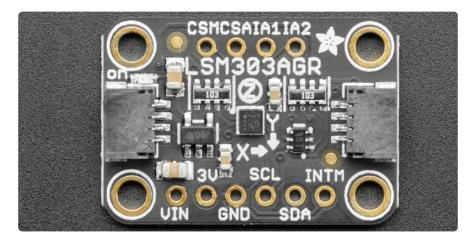
In addition to being a physically smaller and easier to lose chip, there are a few other difference as well. The chip itself exposes an interrupt pin for the magnetometer (INT M) (perhaps a feature of the new magnetometer sensor inside?) as well as chip select pins for both the accelerometer and magnetometer (CSA and CSM respectively).
