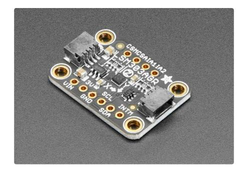
One great feature of the newer LSM303AGR is that it includes a <u>STEMMA QT</u> (https://adafru.it/Ft4) connectors that allow you to use it without soldering. Just plug in a <u>STE</u> <u>MMA QT to male header cable</u> (https://adafru.it/FA-) to connect it to a breadboard or development board with female headers and you're off to the races! You can even chain it with other STEMMA QT breakouts using a <u>STEMMA QT cable</u> (https://adafru.it/FNS)
