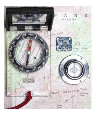
The LSM303 (http://adafru.it/4413) breakout board combines a magnetometer/ compass module with a triple-axis accelerometer to make a compact navigation subsystem. The I2C interface is compatible with both 3.3v and 5v processors and the two pins can be shared by other I2C devices. Combined with a 3-axis gyro such as the L3GD20 (http://adafru.it/1032), you have all the sensors you need for a complete IMU (Inertial Measurement Unit) for use in aerial, terrestrial or marine navigation.
