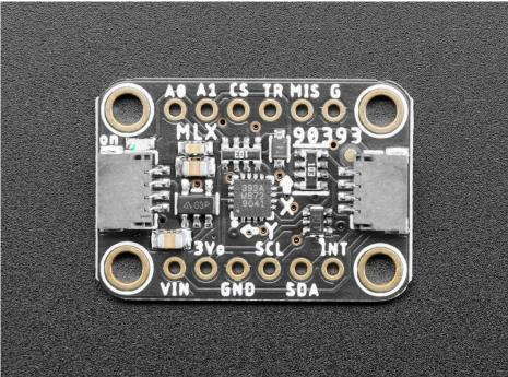
Measure the invisible magnetic fields that surround us, with this wide-range magnetometer. The MLX90393 is a wide range magnetic field sensor, that can measure 16-bits in ranges from +/-5mT up to +/-50mT in all 3 axes.
