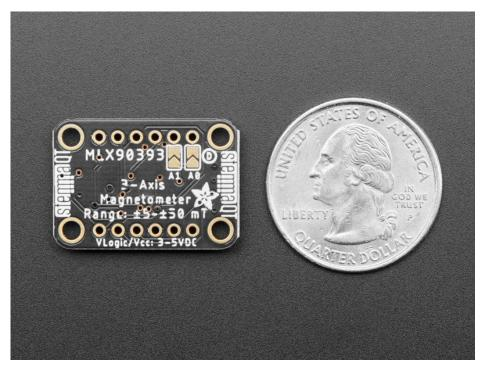
To make it easy to use, we've placed this tiny little sensor onto a breakout board, with a 3.3V power supply and level shifter. This makes it easy to use with any 3 or 5V microcontroller. Our Arduino and CircuitPython code will get you started in a jiffy, with I2C communication to the sensor. You will be readin' out those Gauss's in minutes! With the address select pins you can have up to 4 sensors on one I2C bus.
