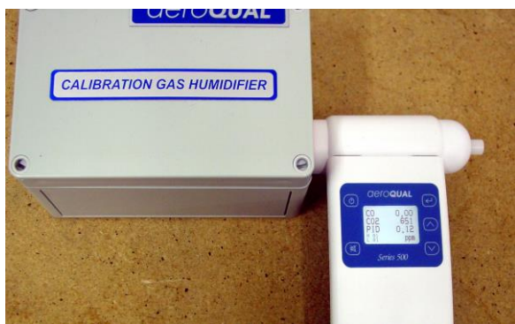
Use this orientation for calibrating PID and CO 2
