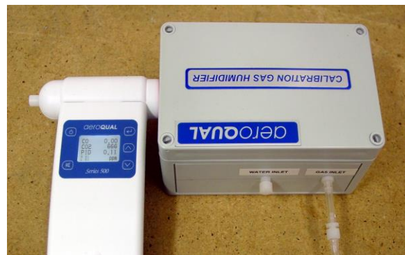
Use this orientation for calibrating CO
