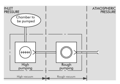
At the pump exhaust, the gases are evacuated to the atmosphere by a roughing pump. Since the MDP compression rate is set by the design, the MDP limit pressure is given by that of the roughing pump used.
