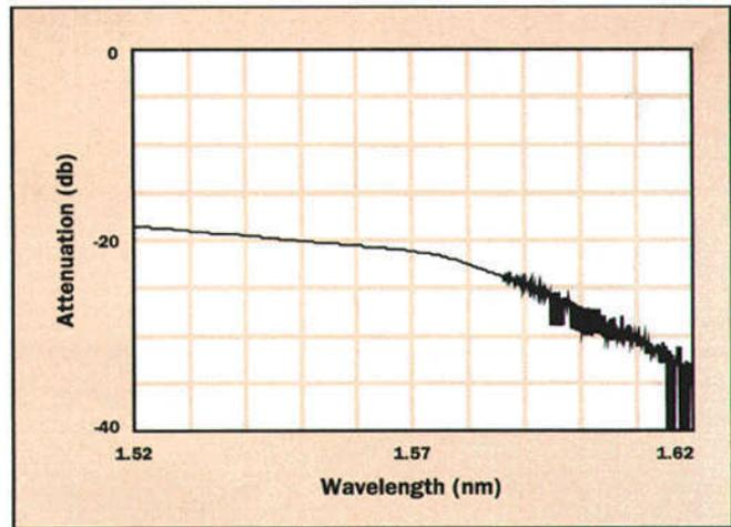
**Figure 8.** Plot of attenuation vs. wavelength representing a monotone decreasing function. The irregular behavior above 1.595  $\mu\text{m}$  is not related to interference of primary mode and reflected components but is most likely due to instrument noise.
