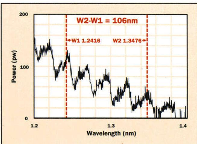
**Figure 4.** Oscillations superimposed on the monotone decreasing loss vs. wavelength function. This plot was obtained from one 0.375-inch loop of a Corning Titan single-mode fiber.
