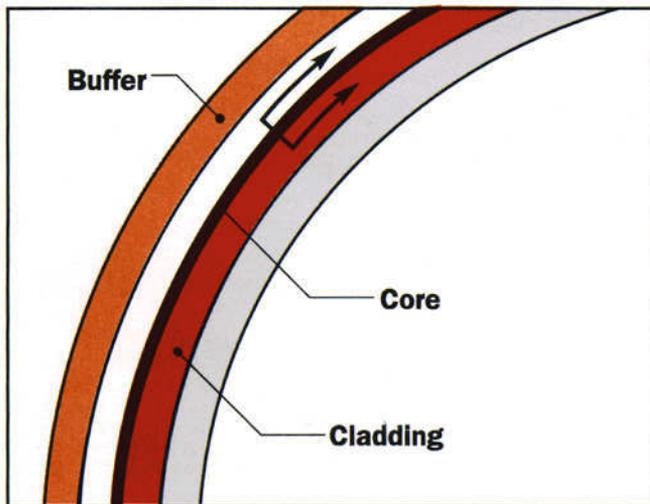
**Figure 1.** Light propagation in a bent single-mode fiber. The outer region of a mode must travel faster than its inner region.
