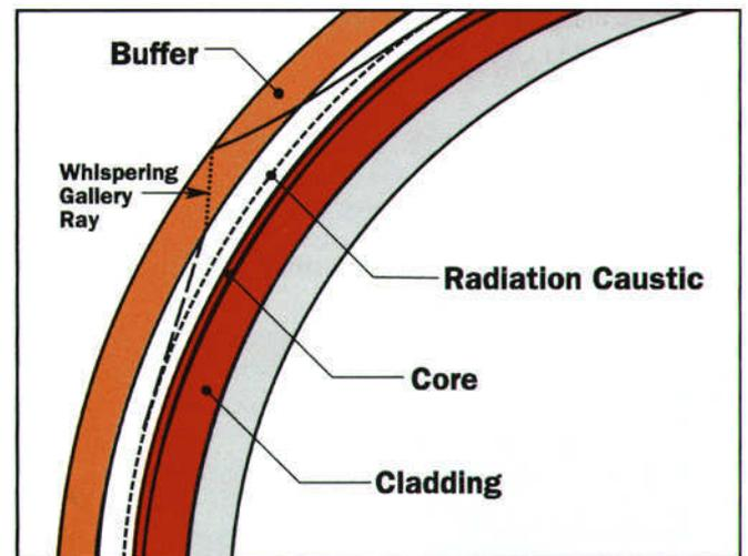
**Figure 3.** Illustration of origin of interference effects caused by light radiated from the core being reflected back into the core.
