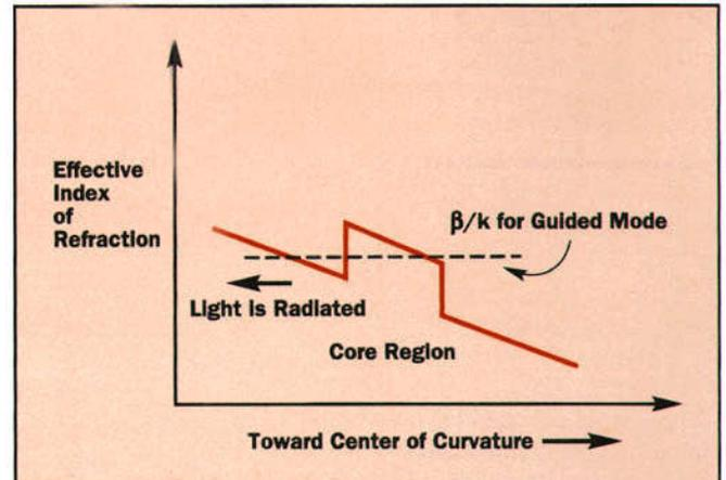
**Figure 2.** Effective index of refraction used to model the effect of fiber bending while assuming a geometrically straight fiber.
