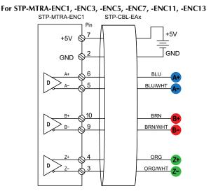
**Optical Encoder Line Driver Wiring Diagram**
