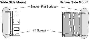
Unless you are running at 1 Amp/phase motor current or below, you may need a heat sink. Often, the metal subpanel being used for the control system will make an effective heat sink.
