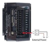
This fuse is not user replaceable. If you want to install a user serviceable fuse in your system, install a fast acting 2 amp fuse in line with the + power supply lead.
