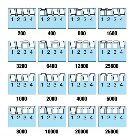
At lower step resolutions such as 200 steps/rev (full step) and 400 steps/rev (half
