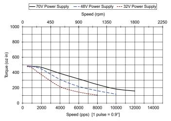
STP-MTRH-34127x Torque vs Speed (1.8° step motor; 1/2 stepping, RMS phase current)
