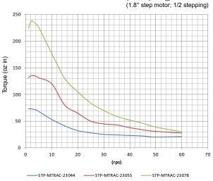
Torque vs. Speed Charts (continued) STP-MTRAC-23xxxx Torque vs Speed @ 340VDC bus
