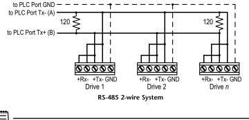
A 120 ohm terminating resistor is required at both ends of a 2-wire network.
