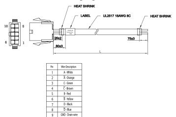
STP-EXT42(H)-xxx Cable Wiring Diagram
