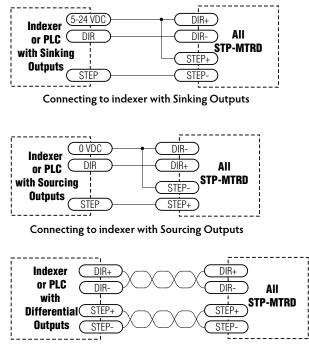
Connecting to indexer with Differential Outputs
