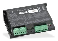
Terminal block part #s (shown) are Phoenix Contact (www.phoenixcontact.com) Both terminal blocks are included in STP-CON-1 for replacement connectors
