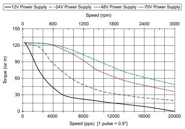
STP-MTRD-23042 Torque vs Speed (1.8° step motor; 1/2 stepping)
