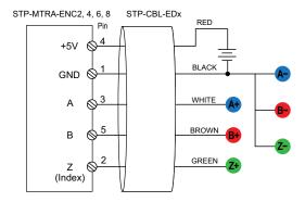
Optical Encoder Single Ended (Push-pull/Totem) Wiring Diagram
