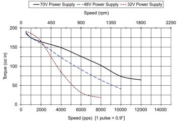
STP-MTRH-23079x Torque vs Speed (1.8° step motor; 1/2 stepping, RMS phase current)
