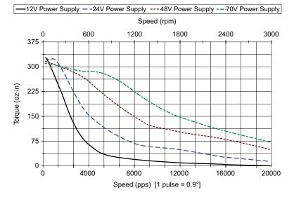
STP-MTRD-24075 Torque vs Speed (1.8° step motor; 1/2 stepping)
