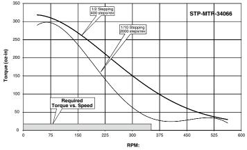
It looks like the STP-MTR-34066 stepping motor will work. However, we still need to check the load to motor inertia ratio:
