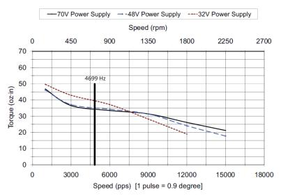
Figure 2: Torque for STP-MTR-17040 at 4.7 kHz
