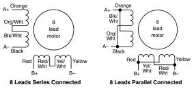
Step motor wire lead colors vary from one manufacturer to another. The example above only pertains to STP-MTRAC-34075(x) and 34115(x) SureStep Motors. For NEMA 42 wire colors, see "Connecting a STP-MTRAC(H)-42 Motor" in Chapter 7.
