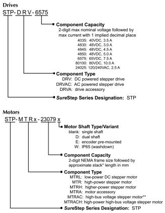
\* The length of the motor that produces torque (not including shaft)
