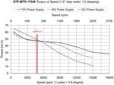
Consider STP-MTR-17048: STP-MTR-17048 Torque vs Speed (1.8° step motor: 1/2 stepping
