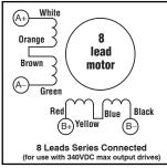
Use the series winding diagram with STP-DRVAC-24025 drives (115 or 230 VAC)
