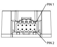
Note: Pin 1 and Pin 2 are internally connected. Pin 7 and Pin 8 are internally connected inside the encoder.
