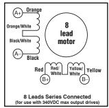
WARNING: Always wire STP-MTRAC motors in series when using the STP-DRVAC-24025
