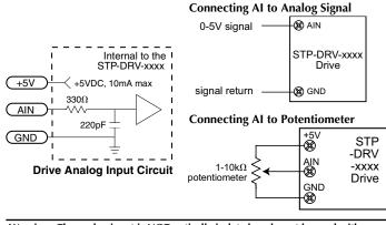
Warning: The analog input is NOT optically isolated, and must be used with care. It may operate improperly and it can be damaged if the system grounds are not compatible.
