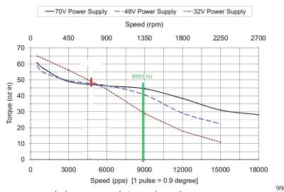
kHz will be approximately 26 oz·in at 32VDC and 44 oz·in at 70VDC. Based on the torque, this motor meets the desired 11.51 oz·in requirement. The rotor intertia, per the motor specification is  $0.45 \text{ oz·in}^2$  or 0.000024 lb·in·sec<sup>2</sup>. Load/Motor inertia ratio:
