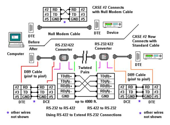
The pin numbers for the RS-422 connections are not shown, they may vary according to the model, but the signal name will be shown on the data sheet.
