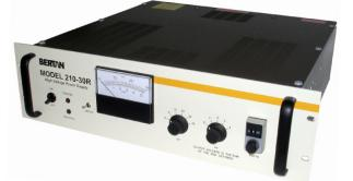
Spellman's Bertan brand of 210 Series of 125 to 225 watt high voltage power supplies provide regulated high voltage outputs from 1 to 50kV. The low noise, linear topology employed results in extremely low output ripple specifications. Units are inherently reversible by design, providing either positive or negative output polarity. The 210 is fully arc and short circuit protected. Excellent regulation specifications are featured along with outstanding stability performance.
