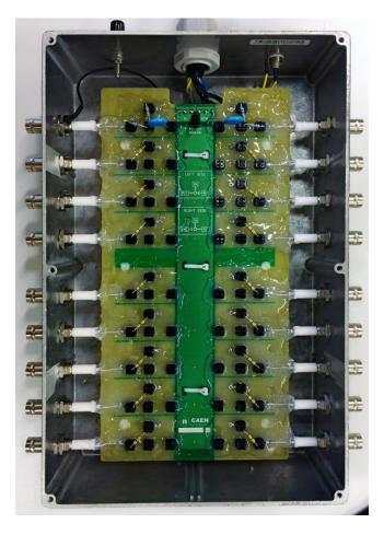
Each output stage can be configured as "direct" or "filtered"; see below: Left side Right side
