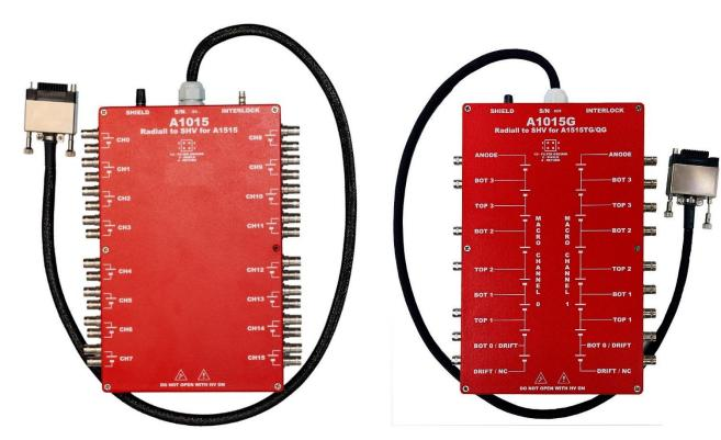
The CAEN A1015G is a 14/16 Stacked Channel Multipin Radiall to SHV connector Adapter for the A1515TG and A1515QG power supply modules; it allows to adapt the Radiall 691803004 type Multipin connector into Radiall SHV R317580-type HV coaxial connectors. Moreover, it is possible to configure the output stages with a RC filter. Please check the internal settings before each use.
