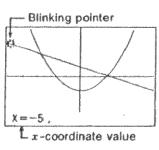
The pointer appears at the extreme left plot of the graph. The key moves the pointer to the right along the graph. Each press of moves the pointer one point, while holding it down causes continuous movement.
