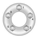
Tighten the wheel nuts firmly in a crisscross sequence, as shown. Notice: Wheel covers will not fit on the vehicle's compact spare. If you try to put a wheel cover on the compact spare, the cover or the spare could be damaged.
