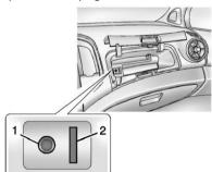
1. 3.5 mm (1/8 in) Auxiliary Input Jack. See Auxiliary Devices on page 7-24.
