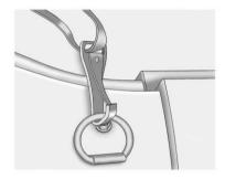
Attach one end of the strap to a cargo tie-down in the rear of the vehicle.
