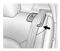
1. Make sure the safety belt is in the retainer hook.
