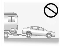
Notice: Towing the vehicle from the rear with the front wheels on the ground could cause transmission damage. Do not tow the vehicle from the rear with the front wheels on the ground.
