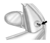
Move the control up, down, or side to side to adjust the mirror.
