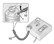
4. Attach the air only hose (10) to the sealant canister inlet valve (1) by turning it clockwise until tight.
