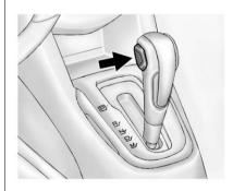
Press the + (plus) end of the button on the side of the shift lever to upshift, or push the – (minus) end of the button to downshift
