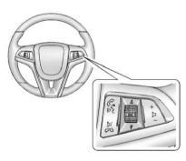
Vehicles with a Hands-Free Phone system can use a Bluetooth-capable cell phone with a hands-free profile to make and receive phone calls. The infotainment system and voice control are used to operate the
