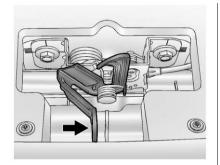
Go to the front of the vehicle and move the secondary hood release lever toward the right side of the vehicle.
