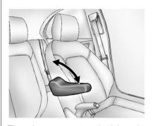
There is an armrest on the inboard side of the driver seat. To raise or lower the armrest, push up or pull down on the armrest.
