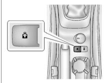
Press at to activate the safety locks on the rear doors. An indicator light comes on when activated.
