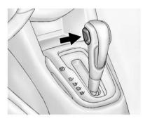
Press the + (plus) end of the button on the side of the shift lever to upshift, or push the – (minus) end of the button to downshift. The Driver Information Center (DIC) in the instrument cluster will change from the currently displayed message to the letter "M," for Manual position, and a number indicating the requested gear.
