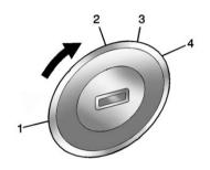
The ignition switch has four different positions.
