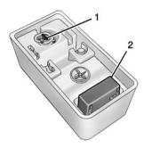
2. Remove the tire sealant canister (1) and the compressor (2).
