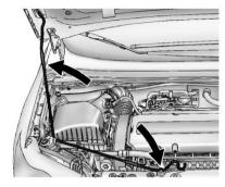
Lift the hood and release the hood prop from its retainer, located in front of the engine compartment. Securely place the hood prop into the slot on the underside of the hood.
