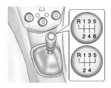
The vehicle may be equipped with a five-speed or six-speed manual transmission.
