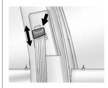
To move it down, press the release button and move the height adjuster to the desired position. After the adjuster is set to the desired position, try to move it down without pressing the release button to make sure it has locked into position.
