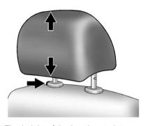
The height of the head restraint can be adjusted. Pull the head restraint up to raise it. Try to move the head restraint to make sure that it is locked in place.
