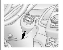
Vehicles with an automatic transmission are equipped with an electronic key lock release system. This system is to prevent ignition key removal unless the shift lever is in P (Park).
