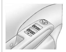
If equipped, push the switch down to open the window. Pull the front of the switch up to close it.
