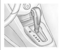
**P (Park):** This position locks the front wheels. It is the best position to use when you start the engine because the vehicle cannot move easily.
