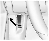
Pull the hood release handle inside the vehicle. It is located on the lower left side of the instrument panel.
