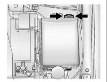
The engine compartment fuse block is on the driver side of the vehicle, near the battery.
