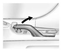
To set the parking brake, hold the brake pedal down and pull up on the parking brake lever. If the ignition is on, the brake system warning light will come on. See *Brake System Warning Light on page 5-15*.
