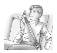
Buckle and position the safety belt as described previously in this section. Make sure that the shoulder belt crosses the shoulder.
