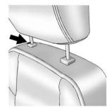
The height of the head restraint can be adjusted. Pull the head restraint up to raise it. Try to move the head restraint to make sure that it is locked in place. To lower the head restraint, press the button, located on the top of the seatback, and push the head restraint down. Try to move the head restraint after the button is released to make sure that it is locked in place.
