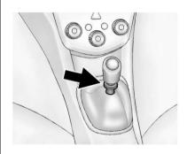
R (Reverse): To back up, press down the clutch pedal, lift up the ring on the shift lever, and shift into R (Reverse). Let up on the clutch pedal slowly while pressing the accelerator pedal.
