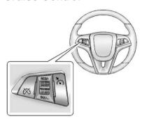
🖰 : Press to turn the cruise control system on and off.
