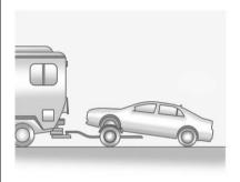
The vehicle can be towed from the front using a dolly. To tow the vehicle using a dolly, follow these steps:
