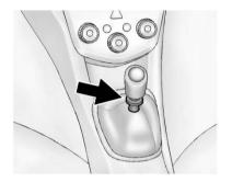
The manual transmission is equipped with a lock ring to prevent shifting into R (Reverse). To shift into R (Reverse), press down the clutch pedal, lift up the ring on the shift lever, and shift into R (Reverse). Let up on the clutch pedal slowly while pressing the accelerator pedal.
