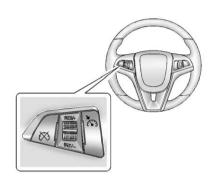
ৈ (On/Off): Press to turn the cruise control system on and off.
