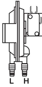
Fig. 3: Without pressure applied to the diaphragm, switch contacts are in the position shown.
