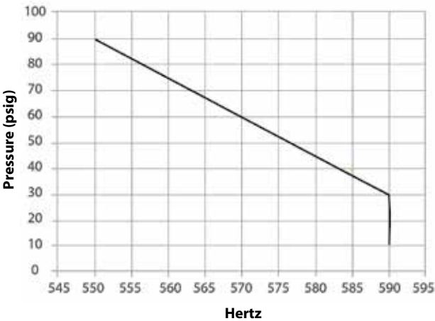
Maximum Step Pulse Frequency vs. Operating Pressure
